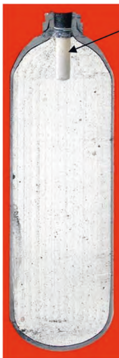
Cross section through an acetylene cylinder showing the "gas space"
