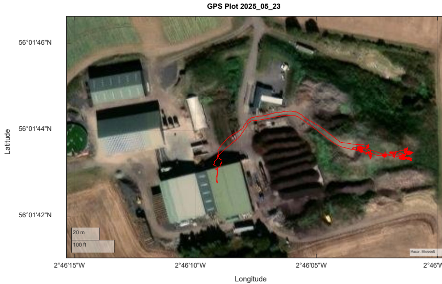
Figure 40: location trace of excavator over one working day
