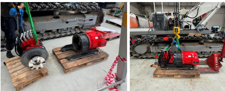
Figure 29: Coupling the pump and electric motor assembly.
