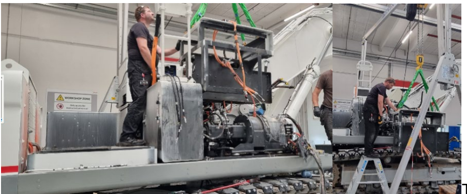
Figure 27: High voltage and pumping compartment removed
