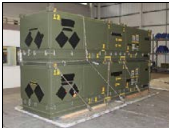
Image 11 - Missile containers restrained to 2 x linked 463L air cargo pallets using chains and tensioners
