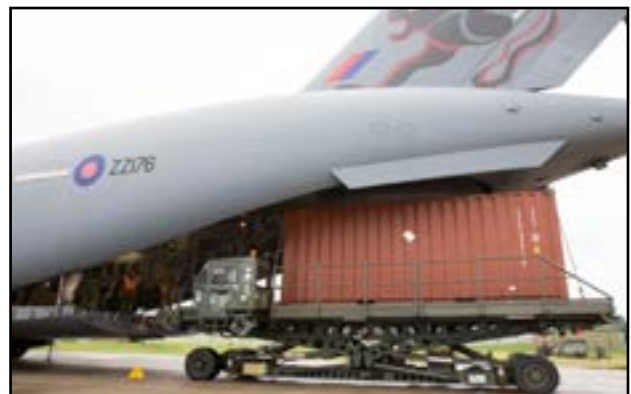
Image 1 & 2 - 20 ft. ISO Container located on 463L air cargo pallets being loaded using an Atlas Transfer Loader.
