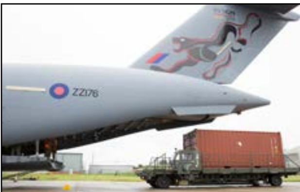
Image 1 & 2 - 20 ft. ISO Container located on 463L air cargo pallets being loaded using an Atlas Transfer Loader.
