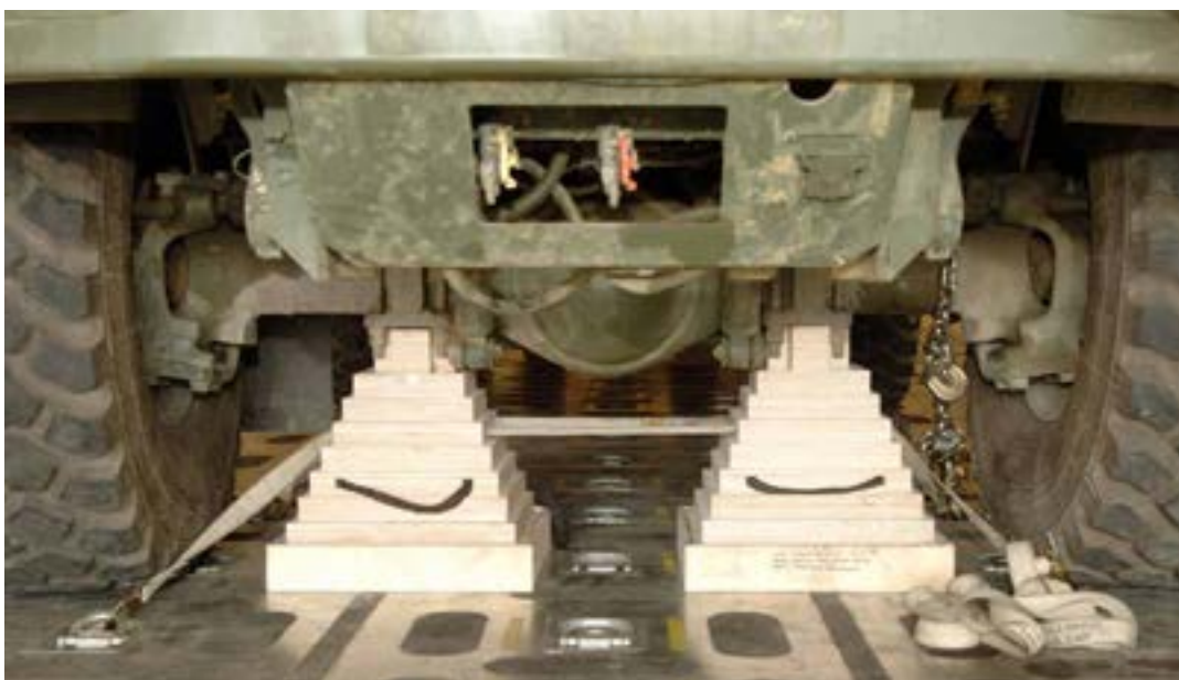
Figure 3 - Front axle sleeper shoring using bespoke sleeper shoring, manufactured from plywood
