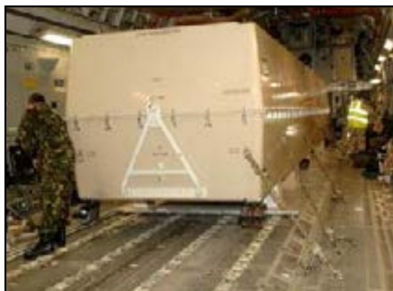
Image 12 - UAV container positioned inside a C-17A - located on linked air cargo pallets, restrained to the aircraft floor from load attachment points on the container
