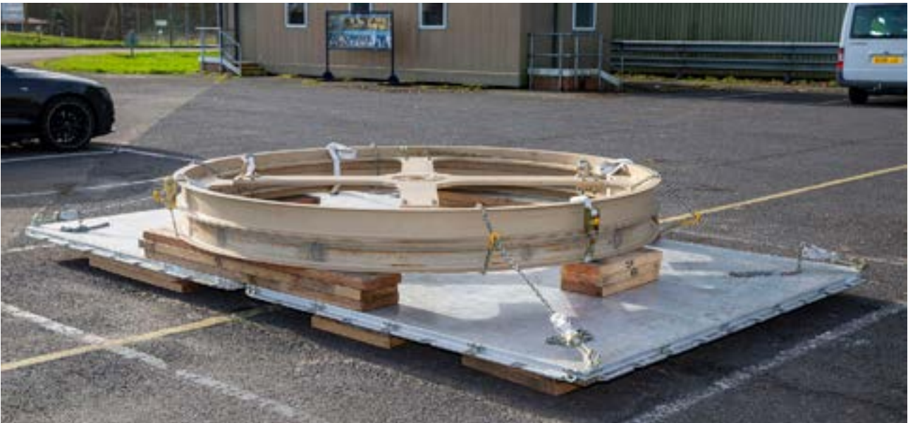
Image 3 - Item secured to 463L Pallet using 5000 lb. chains
