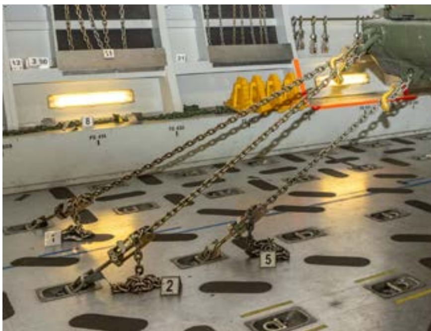
Figure 3 - C-17A – 25 000 lb. Tie down chains and tensioners
