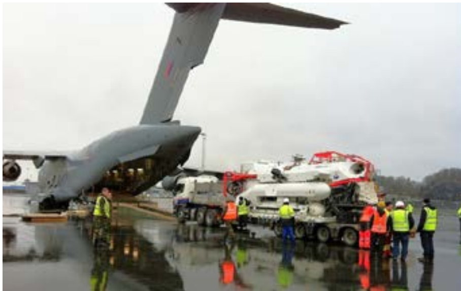
Image 2 - Loading Submarine Rescue Vehicle into a C-17A
