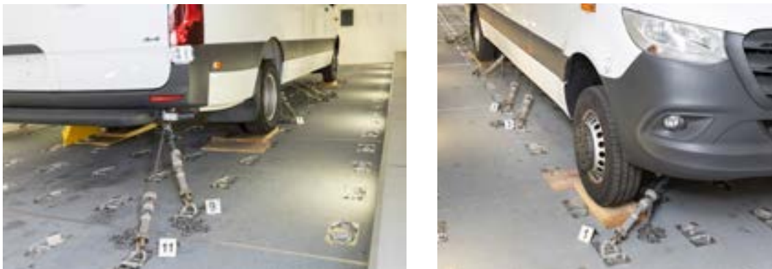
Image 2 - Restraint chains attached to fitted vehicle load attachment points
