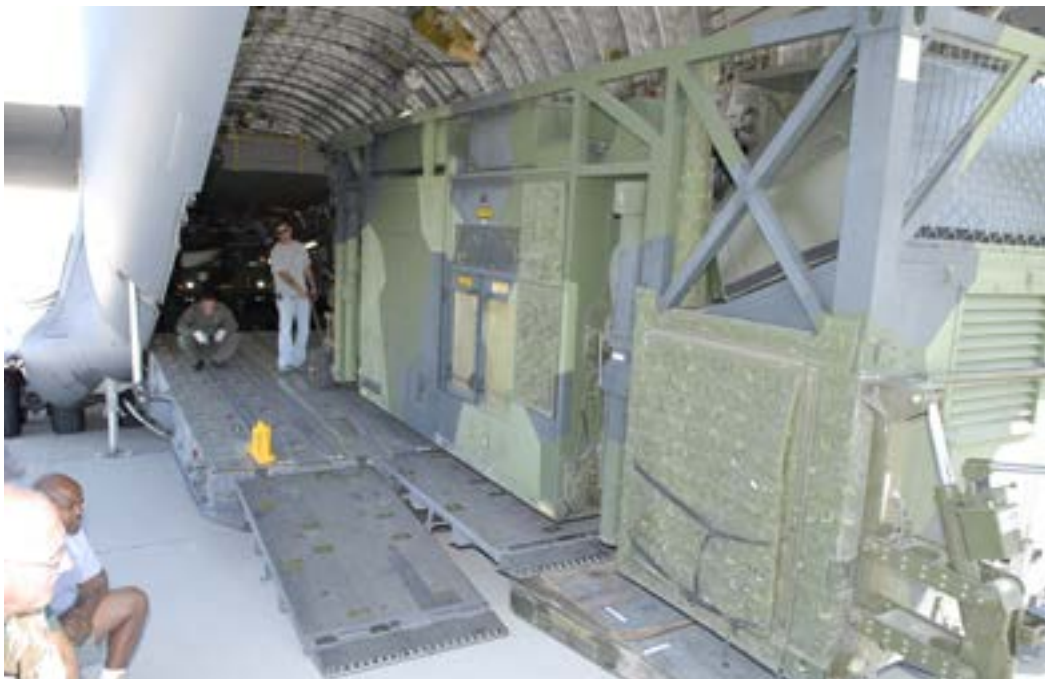
Figure 3 - Cabin on mobiliser wheels winched into a C-17A
