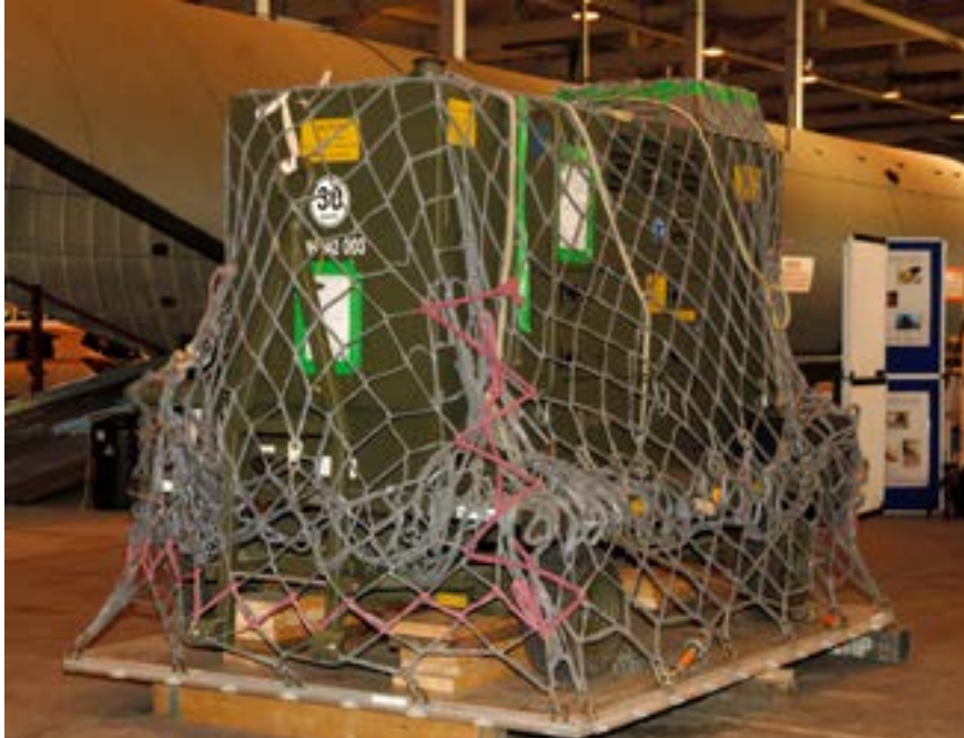
Figure 4 - Palletised trolley - secured to air cargo pallet with an aircraft net
