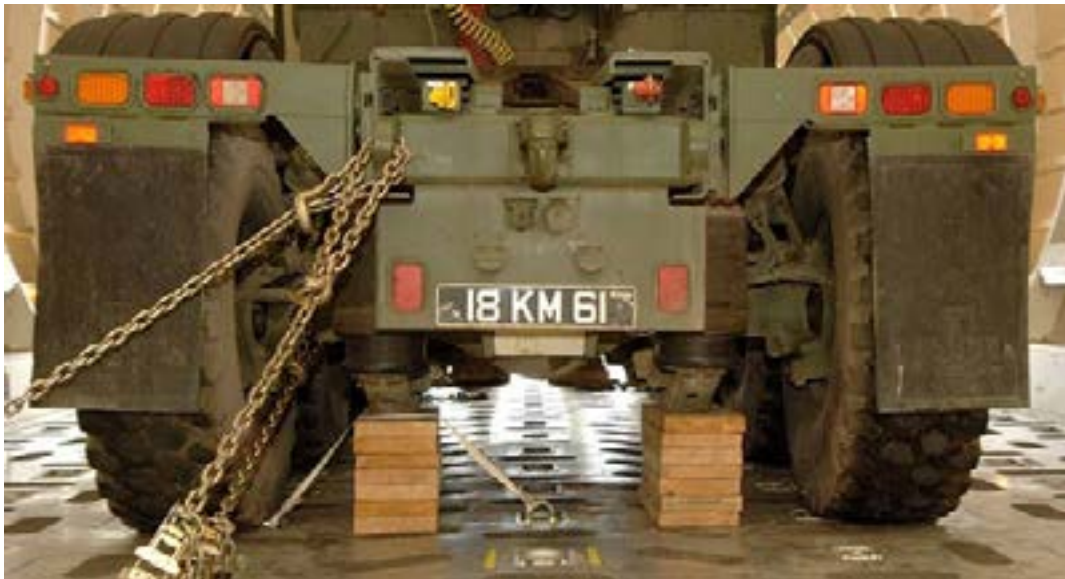
Figure 2 - Rear axle sleeper shoring using standard shoring.
