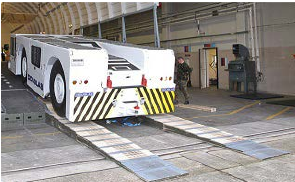
Figure 1 - Approach shoring used to reduce approach angle
