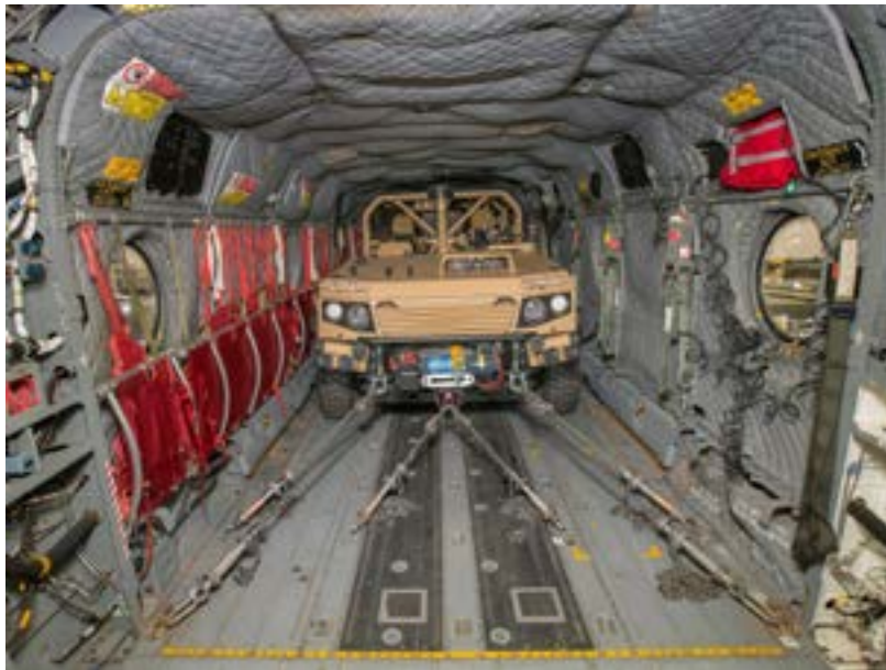
Image 8 - Vehicle restrained inside Chinook HC Mk 6
