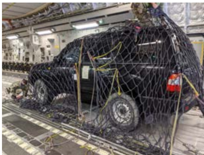
Image 2 - SUV secured by linked Air Cargo Nets to linked 463L Pallets
