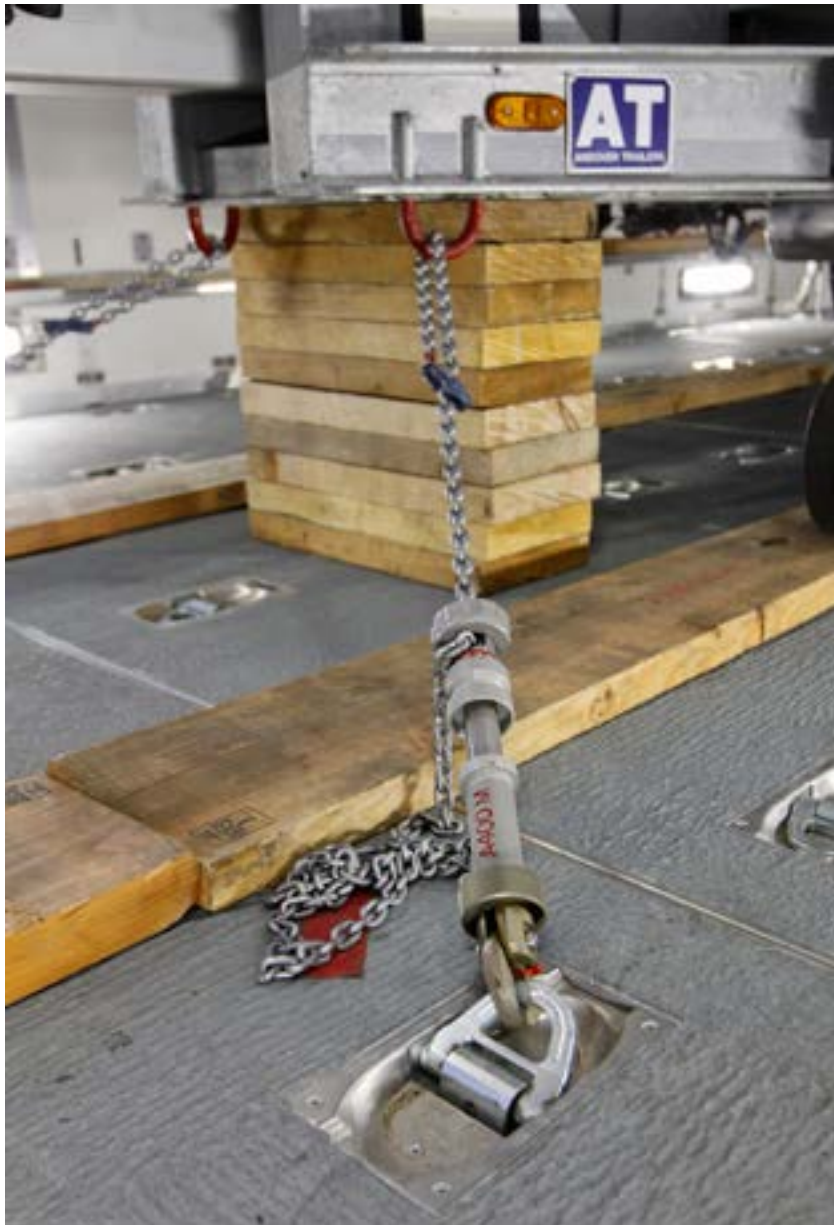
Figure 4 - A400M - 4535 kg. Tie down chain and tensioner
