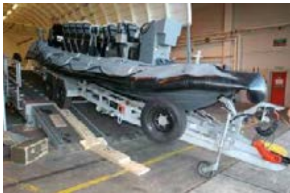
Image 1 - 24 ft. RIB being winched into the C-17A mock-up
