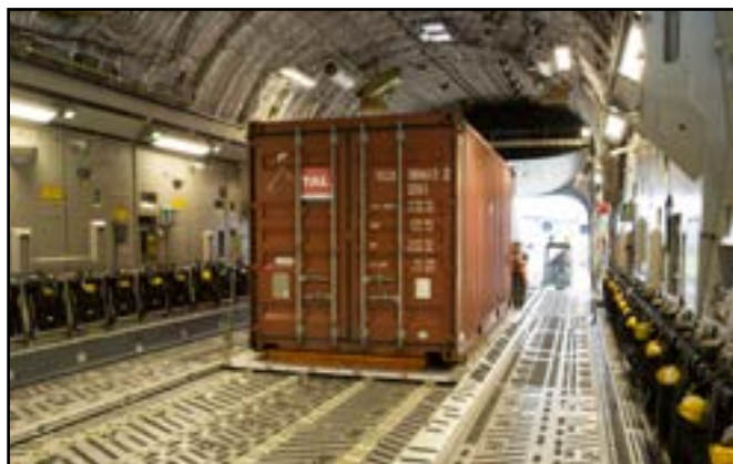
Image 5 & 6 - 20 ft. ISO Container is pushed on, with cabin floor rollers and side guidance in the ADS configuration. The ISO is safety chained to the air cargo pallets at this stage.
