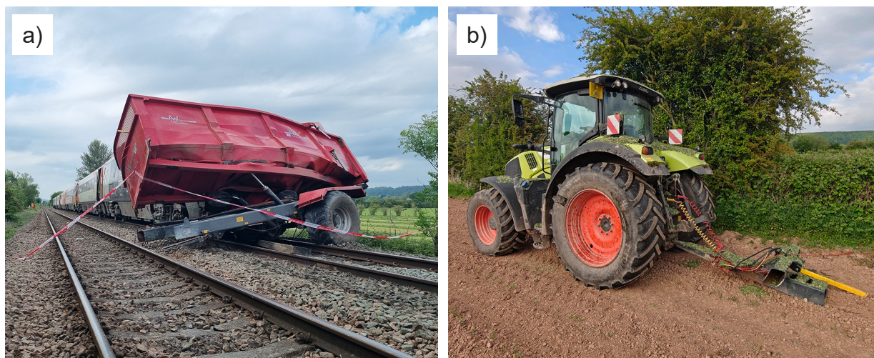
Figure 8: The vehicles after the collision showing a) the train and trailer and b) the tractor.
