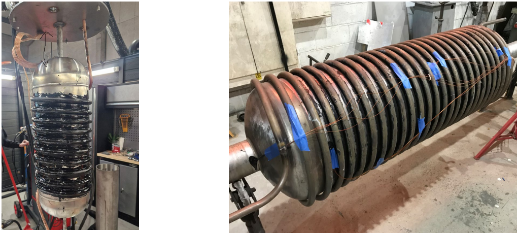
Figure 14 – Prototype (left) and Demonstrator (right) Tank Epoxy
