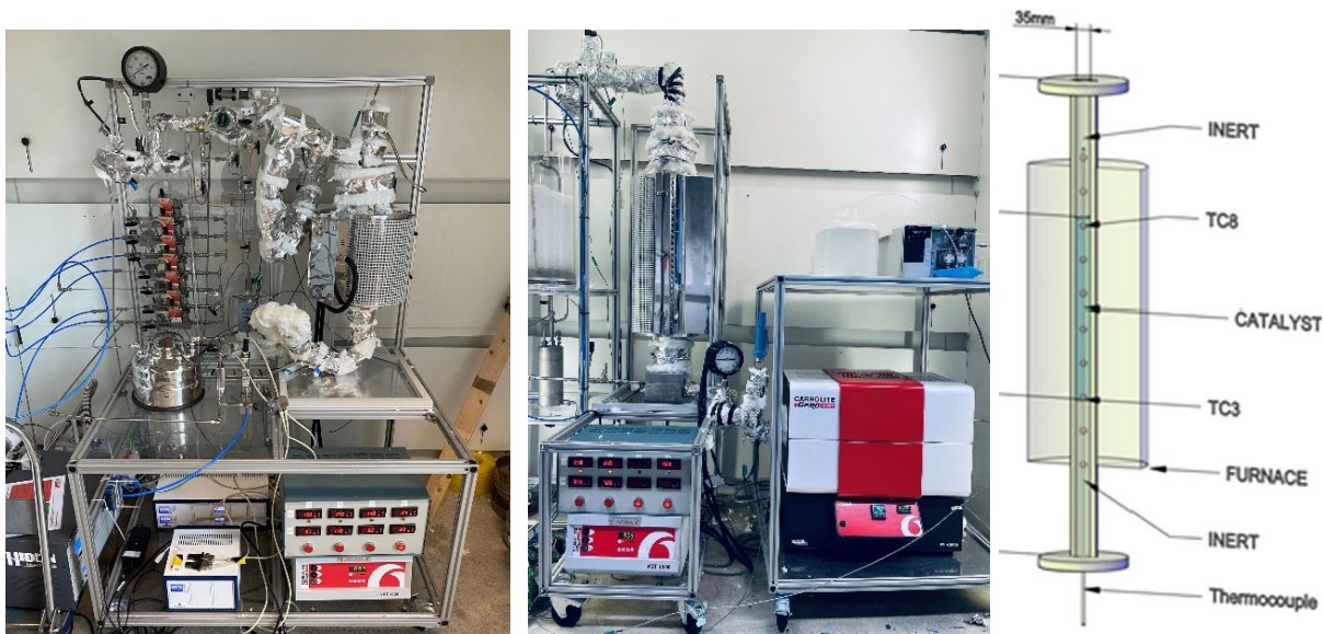
Figure 13: lab scale testing: left) 1-10 grams material development and center) 500 grams reactor testing; right) schematic of the thermocouple location inside the reactor.
