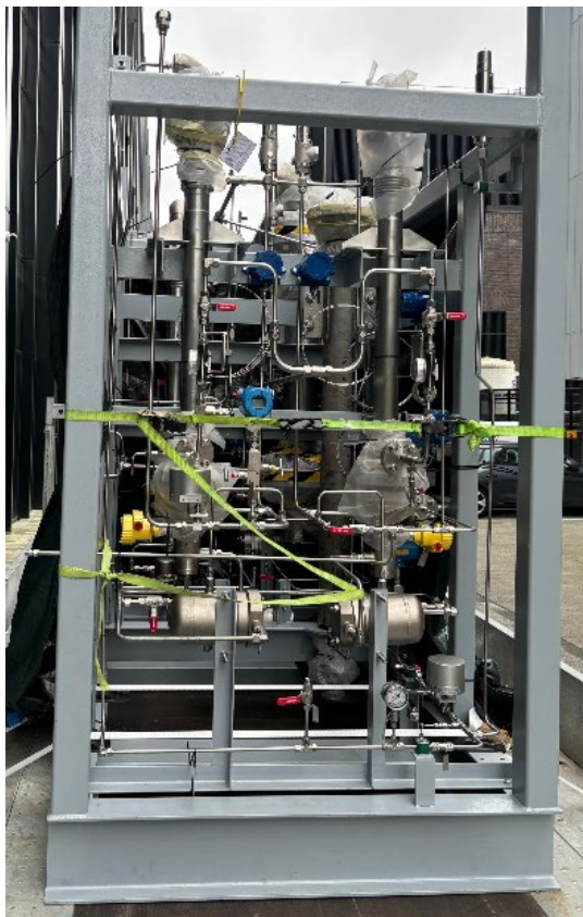
Figure 8: Water gas shift (WGS) reactor skid
