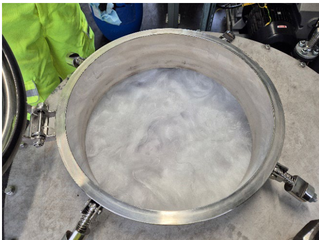
Figure 1. Image of the complete arrangement in the adsorption bed, with glass wool on top of the MOF
