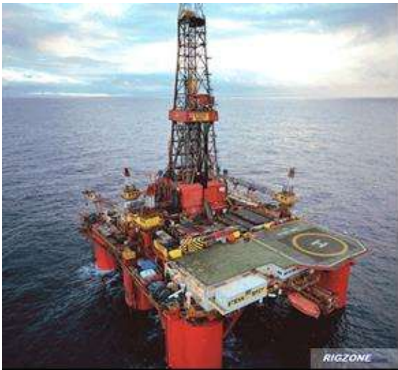
Figure 2-5: Typical semi-submersible rig
