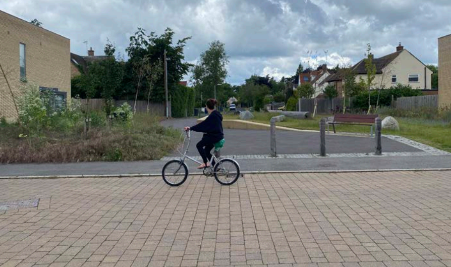
29 Connect to surrounding streets, but filter out motor traffic, and here enhancing the connection point with a pocket park.
