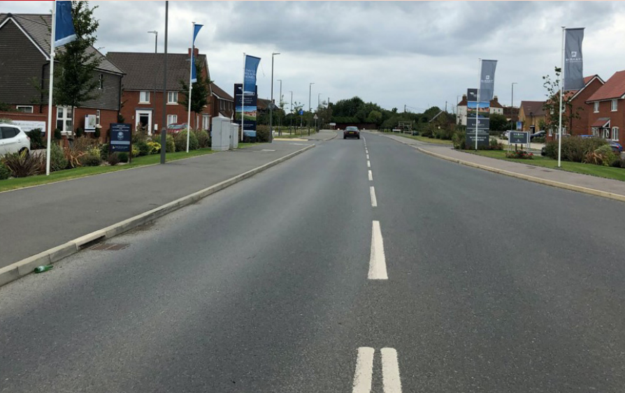
35 Overwide roads, without sufficient enclosure signal to drivers to go too fast, and make the carriageway too hostile for people to cycle on it.
