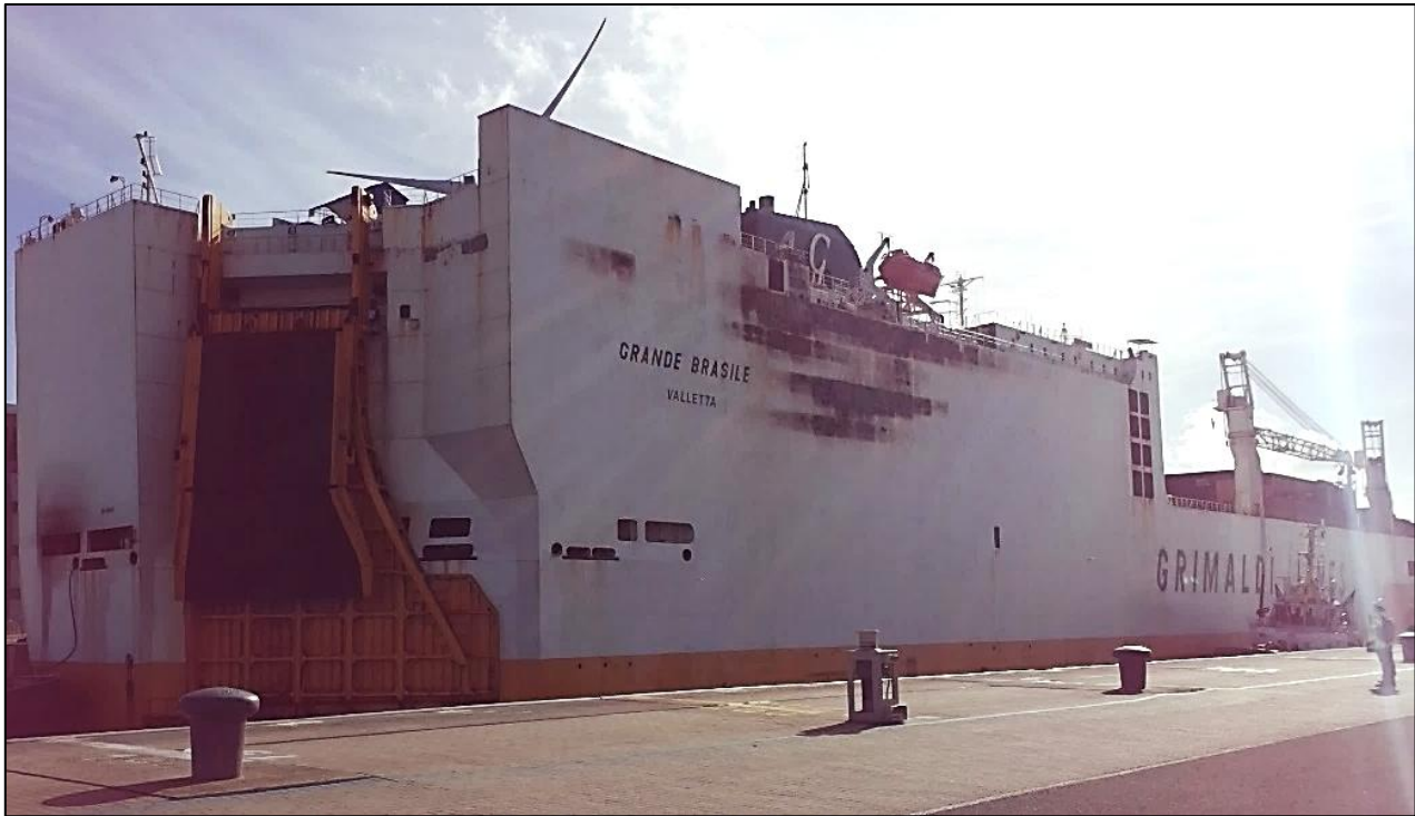
Figure 2: Fire damage visible on the ship's side
