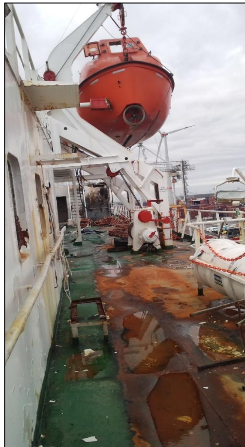
Figure 1: Deformed and scorched deck plating resulting from heat damage
