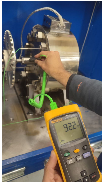
b) Temperature at shaft end (92.2 °C)
