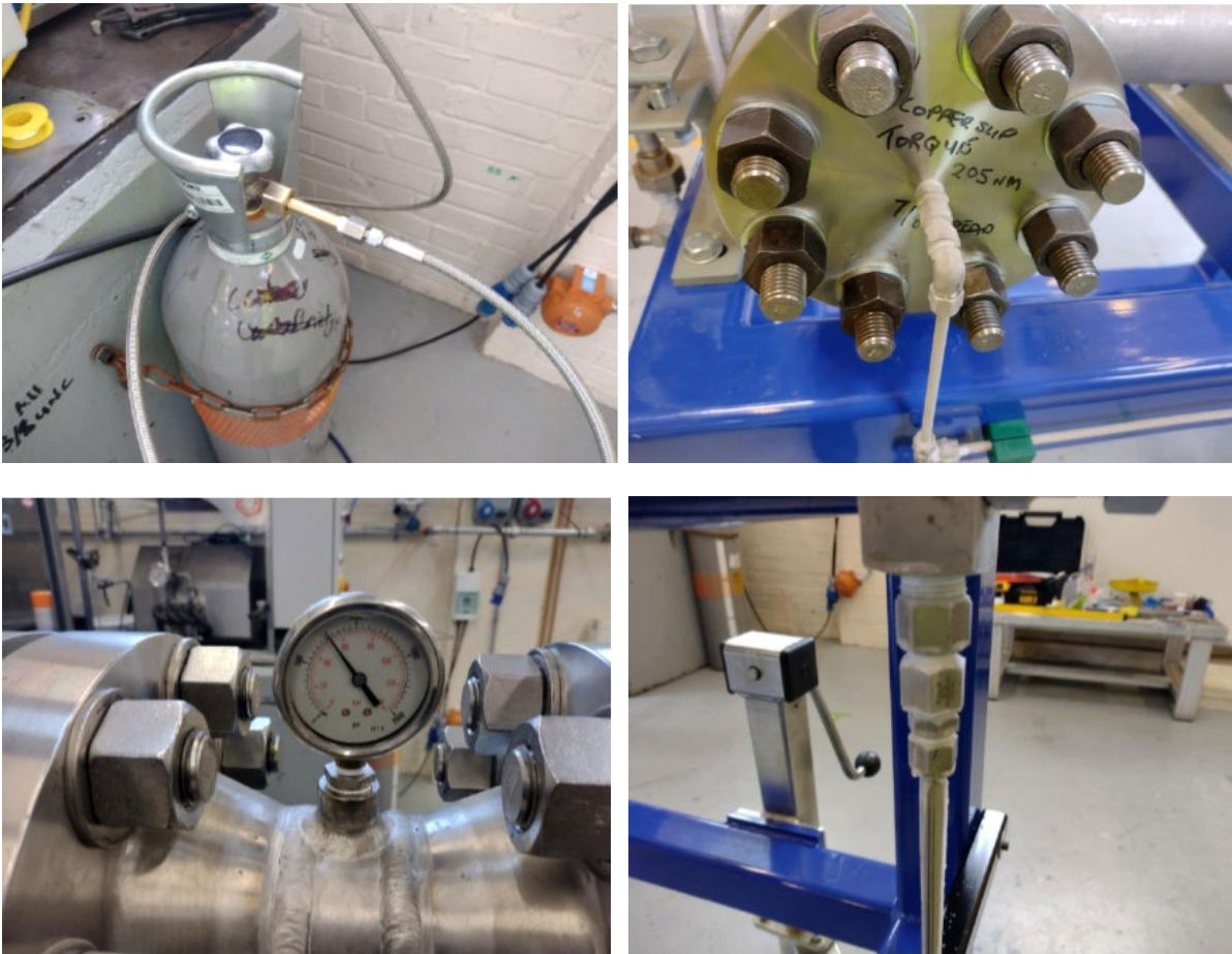
Figure 4: Leak and pressure testing of subassembly 1 and dummy test cell
