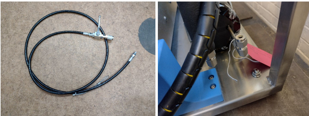
Figure 5: High pressure hose (left), condenser feed connection (right)
