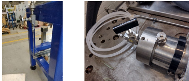
Figure 8: Needle valve vessel 20-l (left), needle valve vessel 1.25-lt (right)
