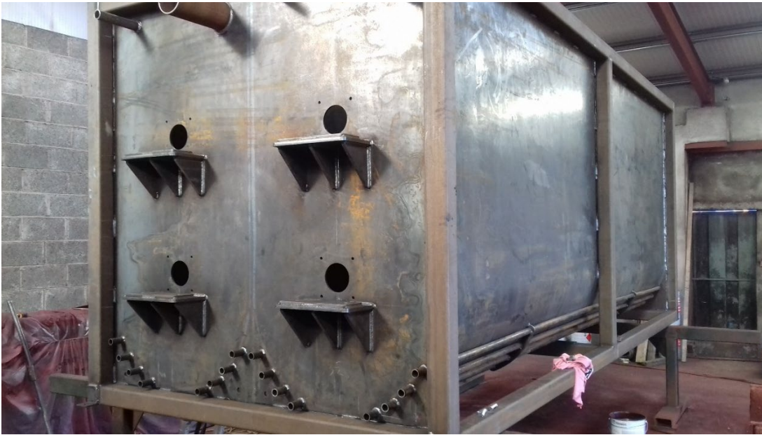
Figure 34: Heavy tank structure with lightweight framing
