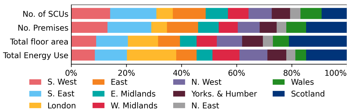
Figure 3.2-2: Regional distribution by SCU and premises count, floorspace and total energy demand
