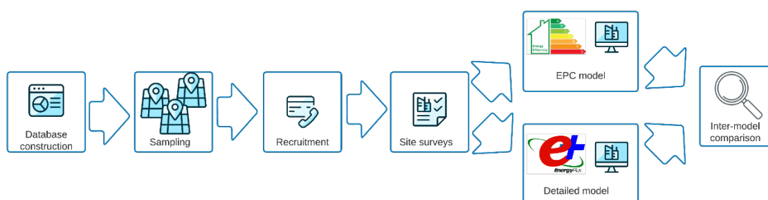
Figure 4-3: Flowchart showing audits and simulation workflow to compare EPCs against bottom-up modelling
