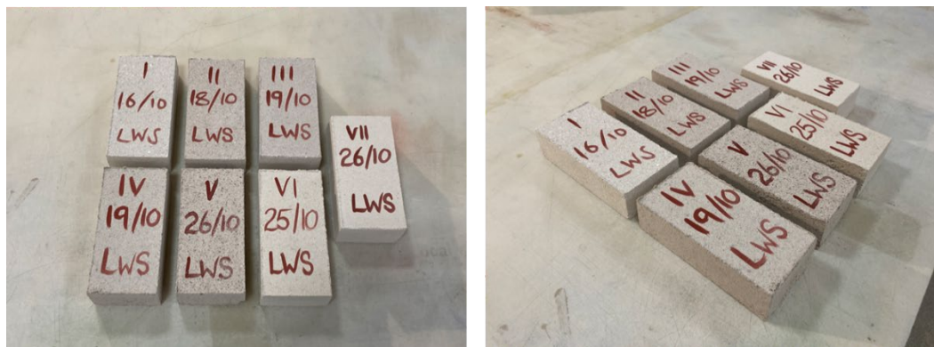
Figure 2.4 – Specimens for testing, made with a range of brick and block mix designs.
