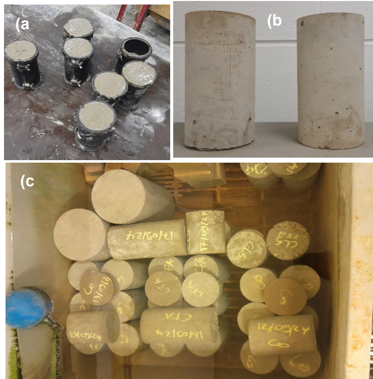
Figure 1. Concrete sample in the mould (a) after demolding (b) and in the water curing tank (c).
