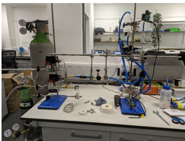
Figure 6: A picture of the in-house-built breakthrough rig.
