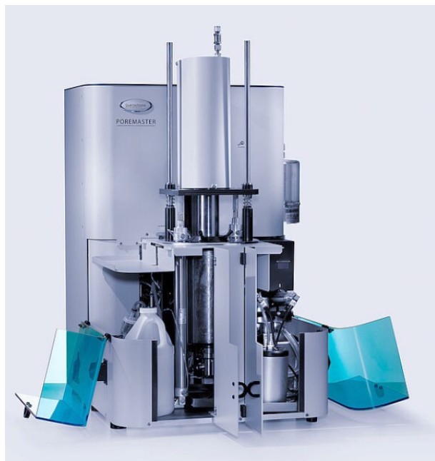
Figure 4: A picture of the Hg porosimeter that are used for the analysis of the m-MOFs.
