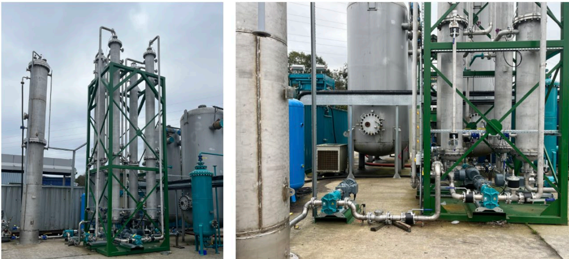
Figure 8 a & b - Carbon capture in the CO 2 Scrubbing Skid
