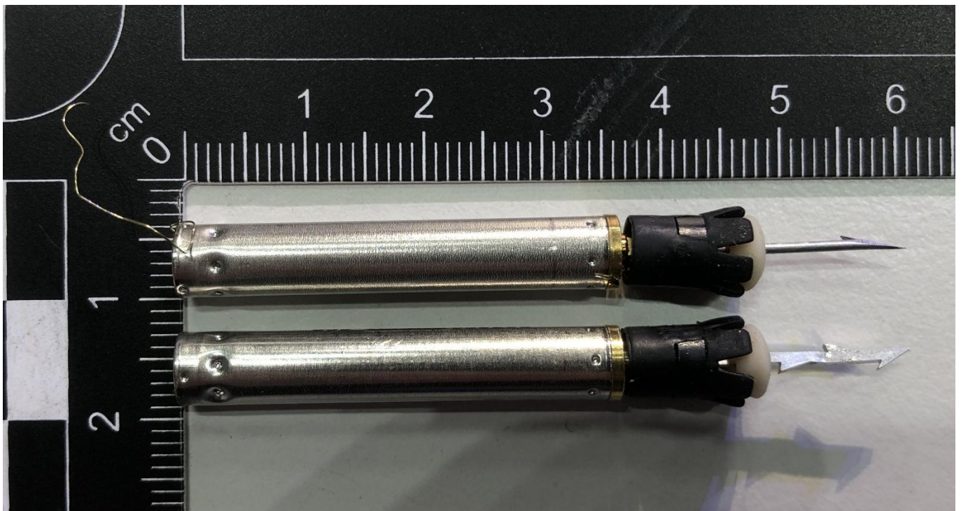
Figure 1: A comparison of the New and Old spear designs. Top: diagram from Axon documentation. 5 Middle: Photograph taken during testing with the Old design on the left and New design on the right. Bottom: Photograph taken during testing with the Old design on the top and the New design on the bottom. Note that the photographs are of probes previously fired into a target as part of accuracy testing, with the spears subsequently straightened out manually, which is the result of any slight misalignments of the spears or impact absorbers.
