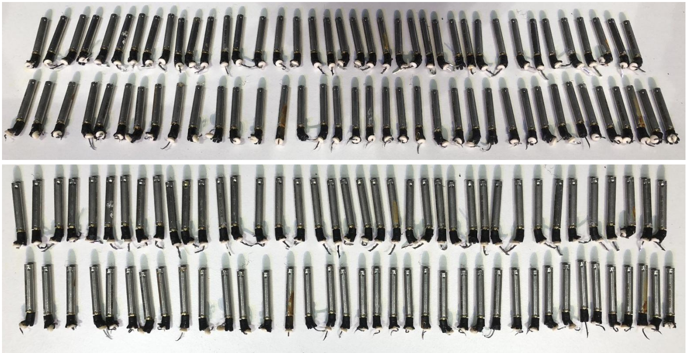
Figure 2: Photographs of the probes used for skull penetration testing, showing the amount and variation of the spear deformation due to impact with the bone. In both photographs (which show different angles of the same arrangement of probes), the top row of probes have the New spear design and the bottom row have the Old design.
