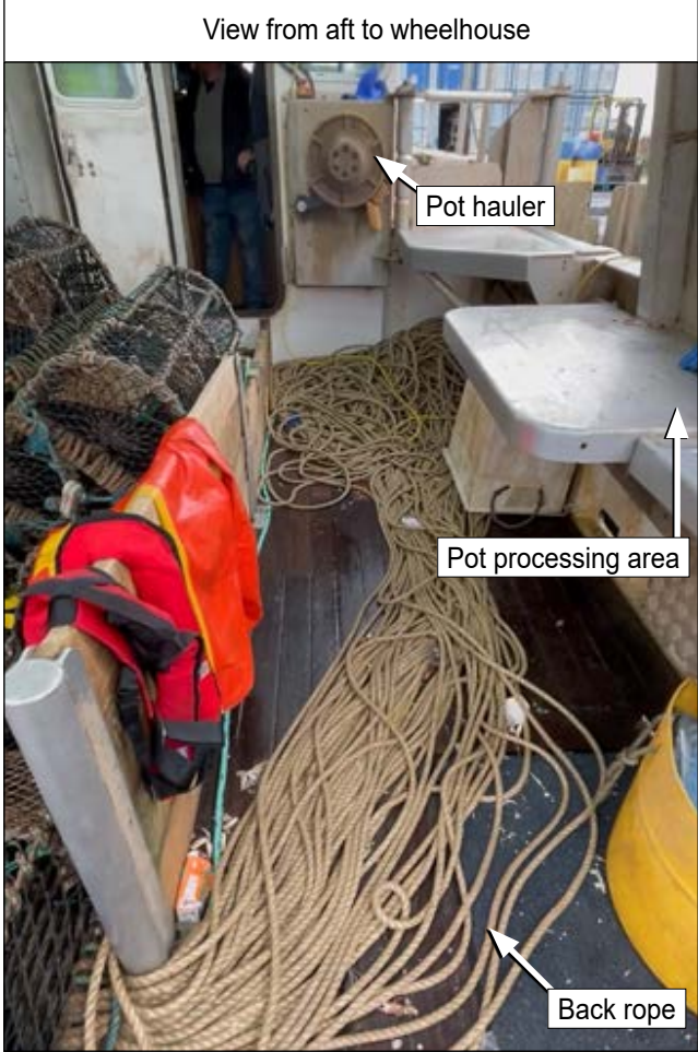
Figure 2: Weston Bay's working deck layout
