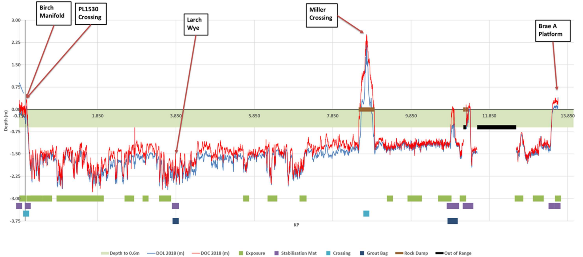
PL1164 Control / Chemical Umbilical Burial Profile
