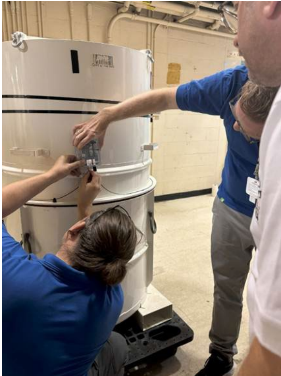
Figure 2. 'Host' facility staff applying an electronic seal to a container under the supervision of an 'Inspector'
