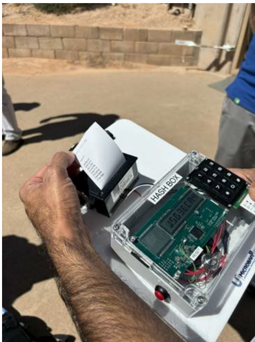
Figure 3. Generation of cryptographic hash message for image verification (used to allow trustable review and redaction of image data)
