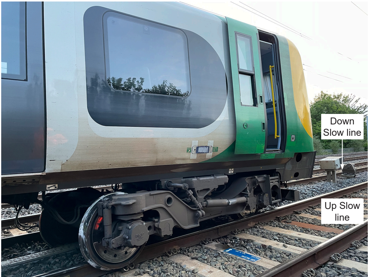
Figure 14: The front of the derailed train.
