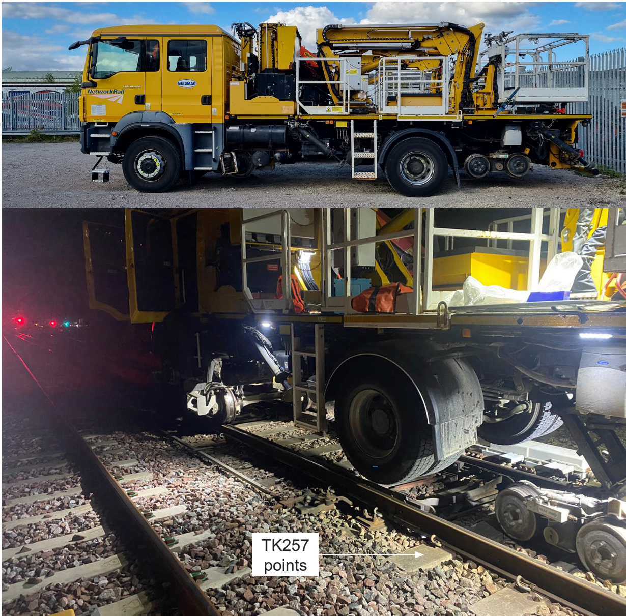
Figure 9: The road-rail vehicle type that ran through TK257 points and derailed (lower image courtesy of Network Rail with RAIB annotations).
