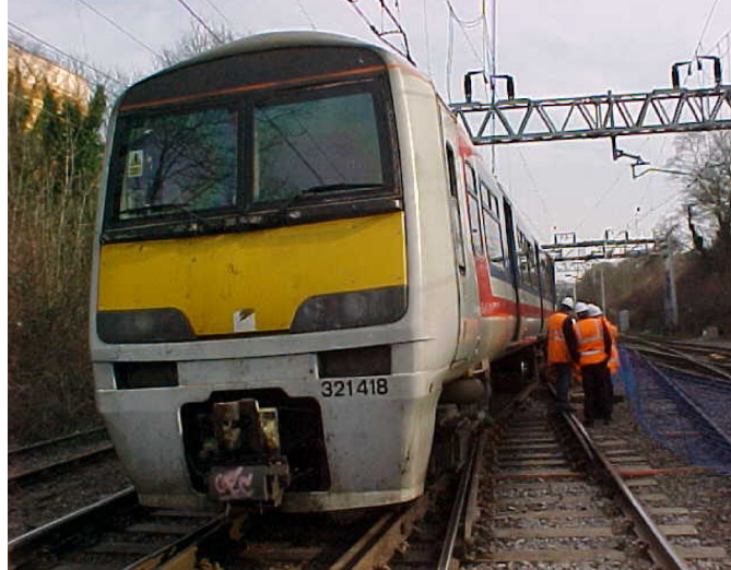
Figure 22: Derailed train on switch diamond points at Hemel Hempstead South Junction (courtesy of Network Rail).
