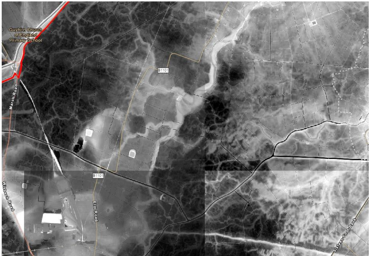
Figure 11: LiDAR extract displaying roddons of varying size and scale, located south-east of Guyhirn adjacent to the western catchment boundary.
