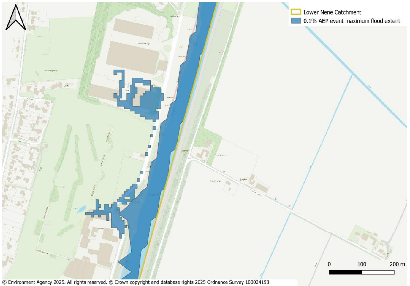
Figure 26: 0.1% AEP event flood extent at Sutton Bridge
