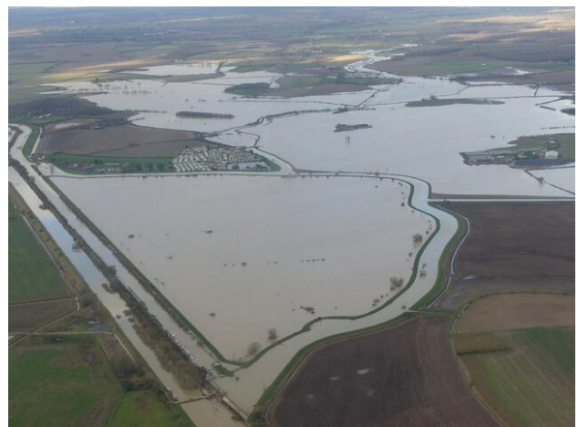
Branston Island flood storage area in operation in 2024 © Simon Tomson. Licensed for reuse under the Creative Commons Licence.
