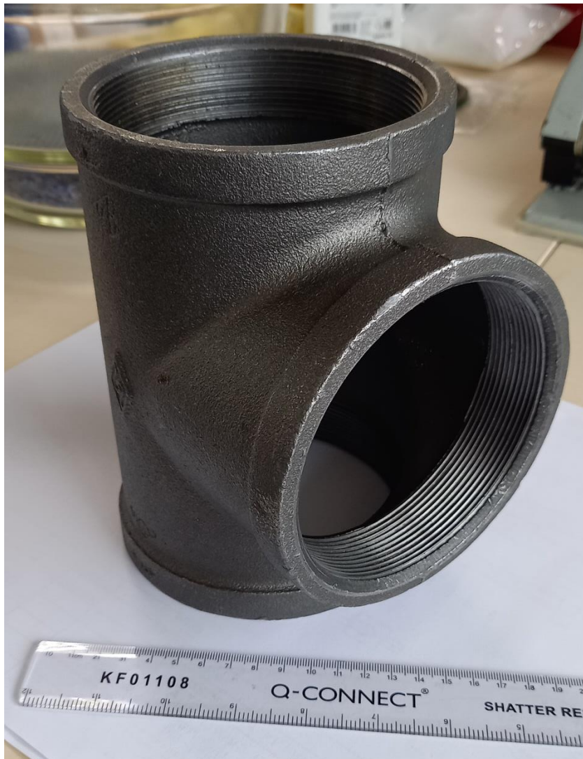
Figure 1 Photograph of malleable iron tee piece on arrival at TWI, note scale indicated by cm ruler.
