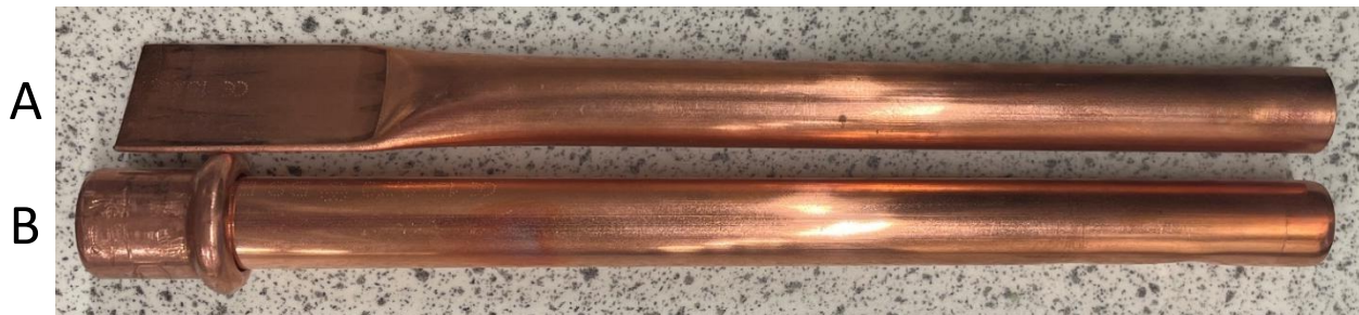
Figure 3.2 – A – Flattened, crimped pipe sample, B, round pipe sample, with gas a certified end cap.
