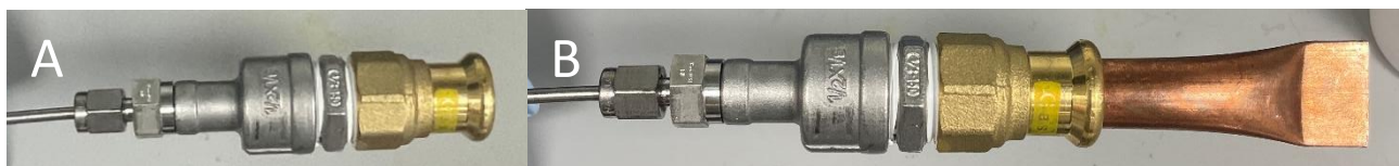
Figure 3.7 – Gaseous hydrogen filling setup with hydrogen gas line adapted to a 15 mm press fitting used to fill samples. A, push it adapter. B, a pipe in the put fit adapter with the protruding end crimped flat.
