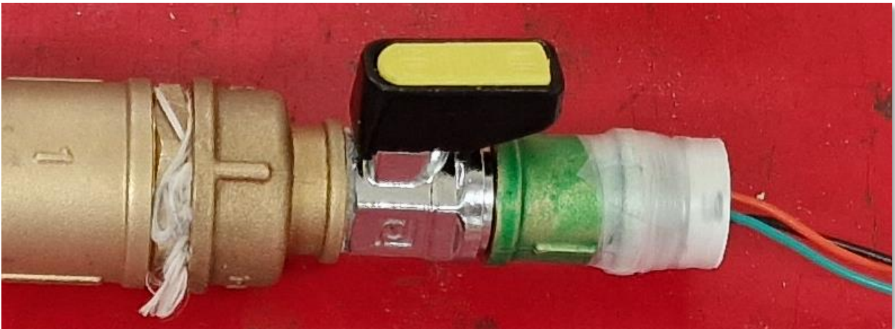
Figure 26: VQ456MR hydrogen sensor attached to a test string
