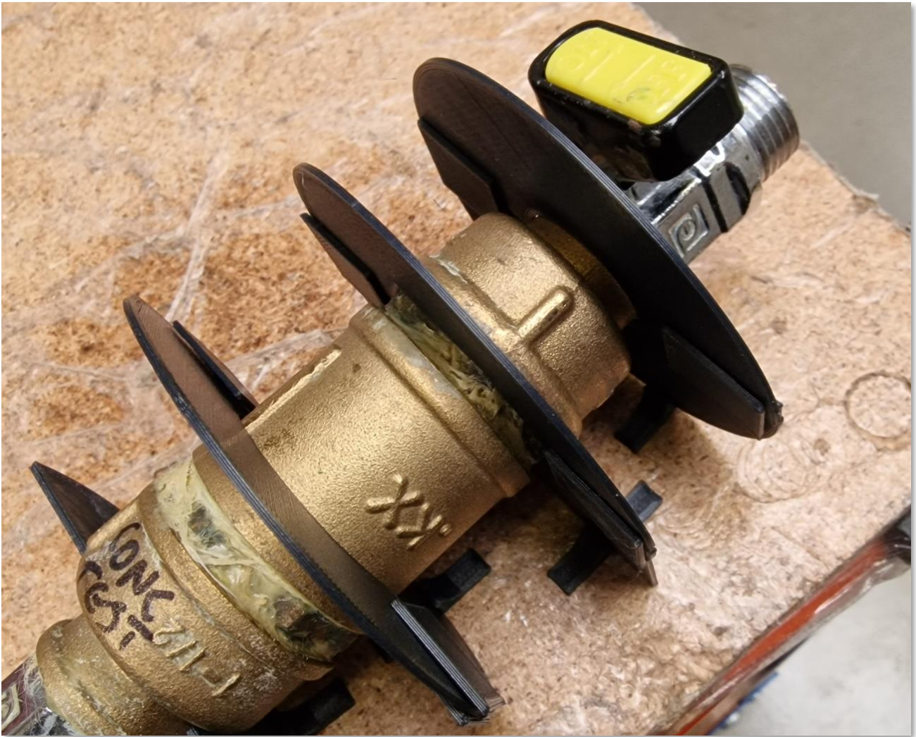
Figure 24: Baffles to aid locating leaks
