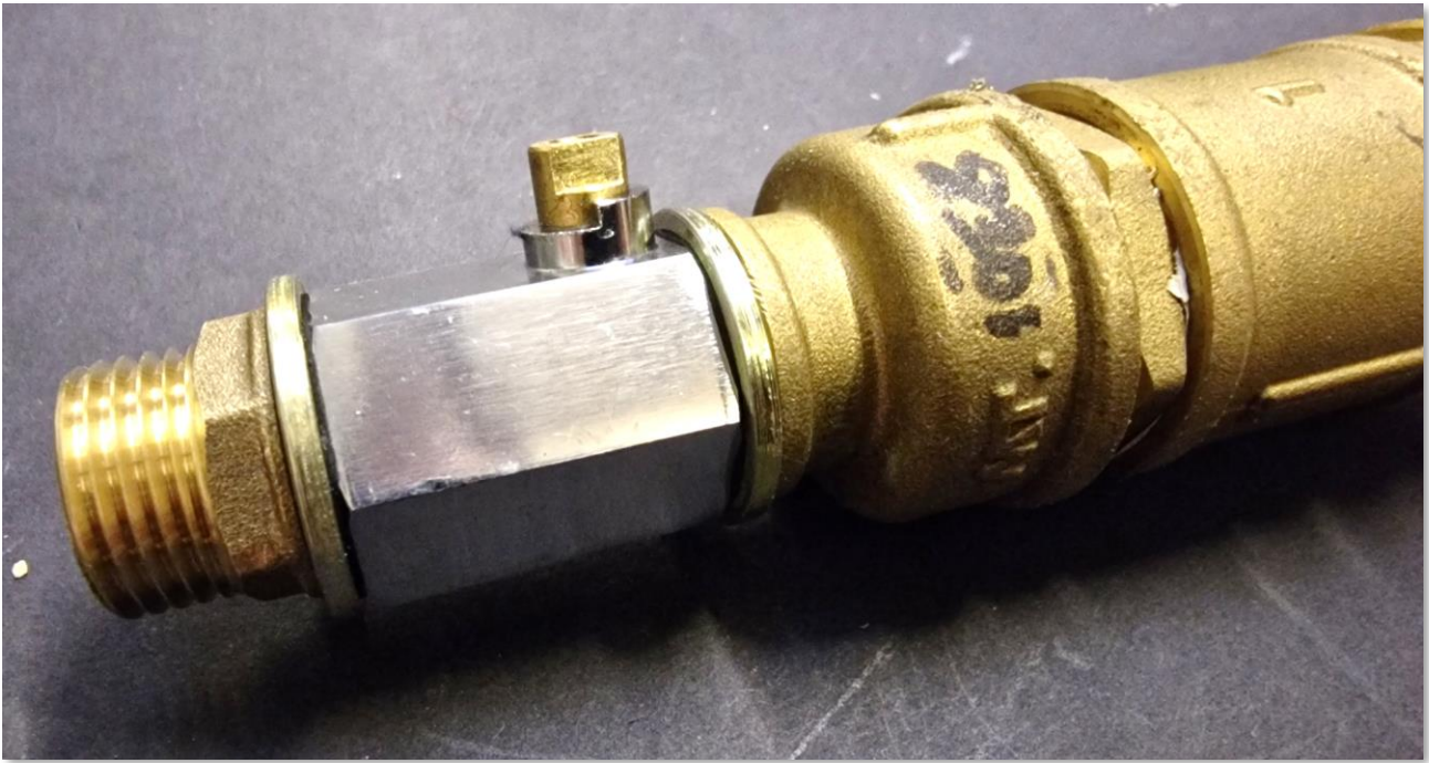
Figure 38: Replacement valve with bonded washers
