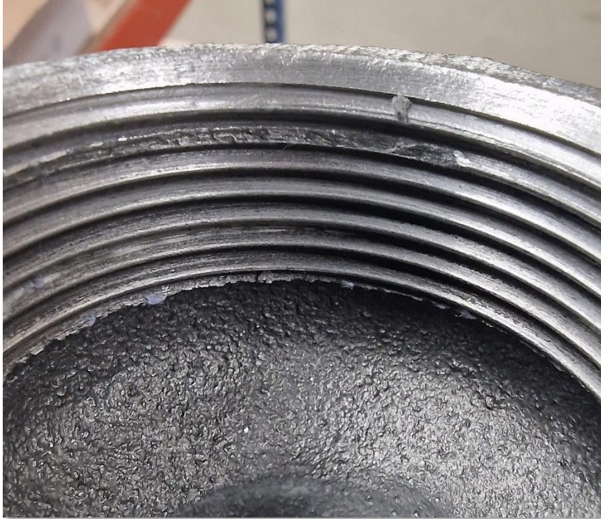
Figure 4: Rough threads on a malleable iron female reducer
