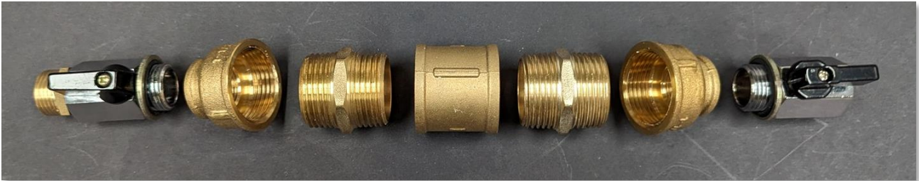
Figure 3: String of 4 test joints
