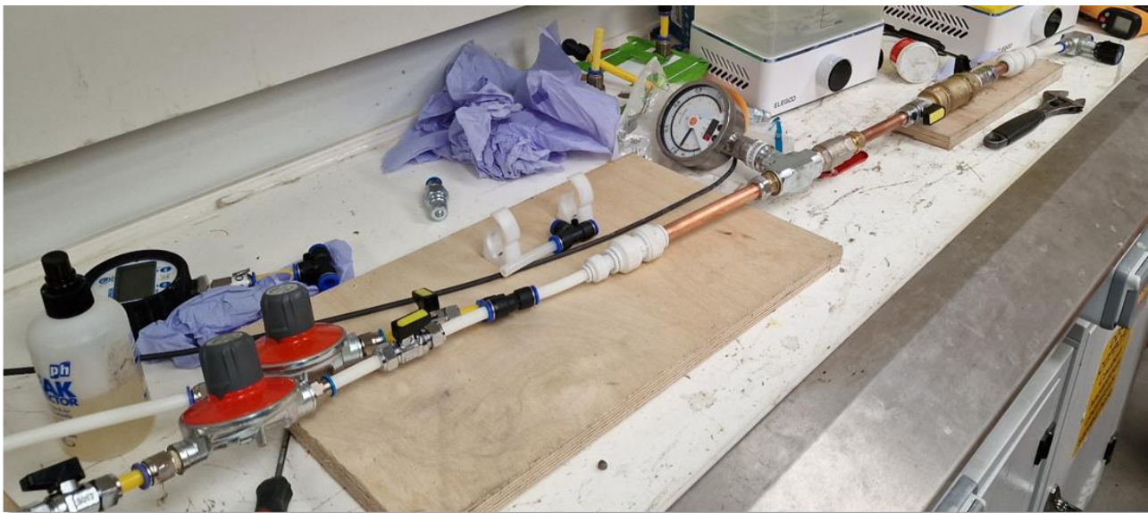
Figure 18: Test setup with twin hydrogen supplies
