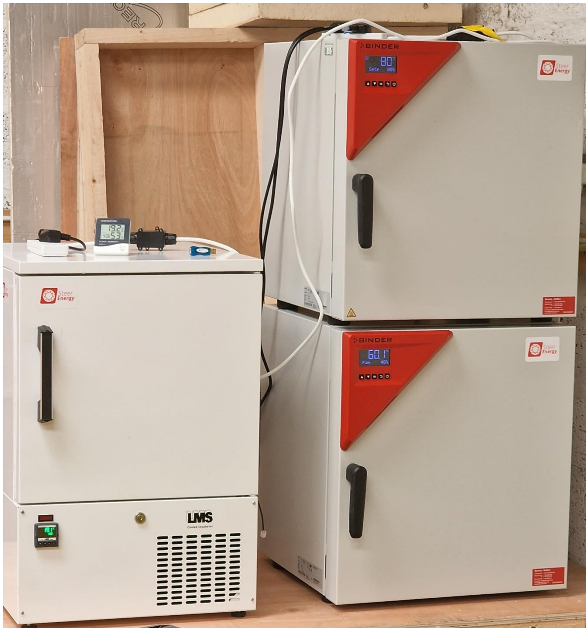
Figure 14: Laboratory ovens and incubator for maintaining consistent temperatures
