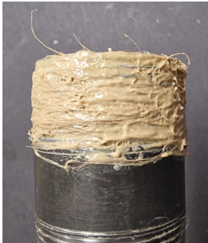
Figure 1: Hemp and compound on a 1 1/2" black steel pipe thread
