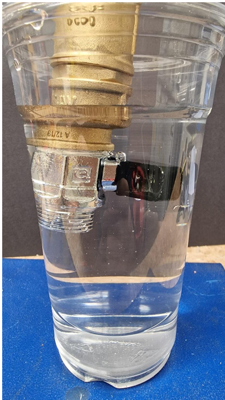
Figure 22: Submerged valve connection
