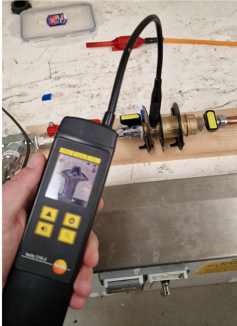
Figure 25: Refined method for identifying leaking threads
