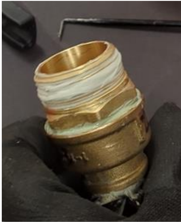
Figure 42: Application of PTFE cord to retired joint B of string 2202-3
