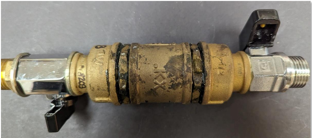
Figure 70: 8203 non-hardening sealant that cured hard
