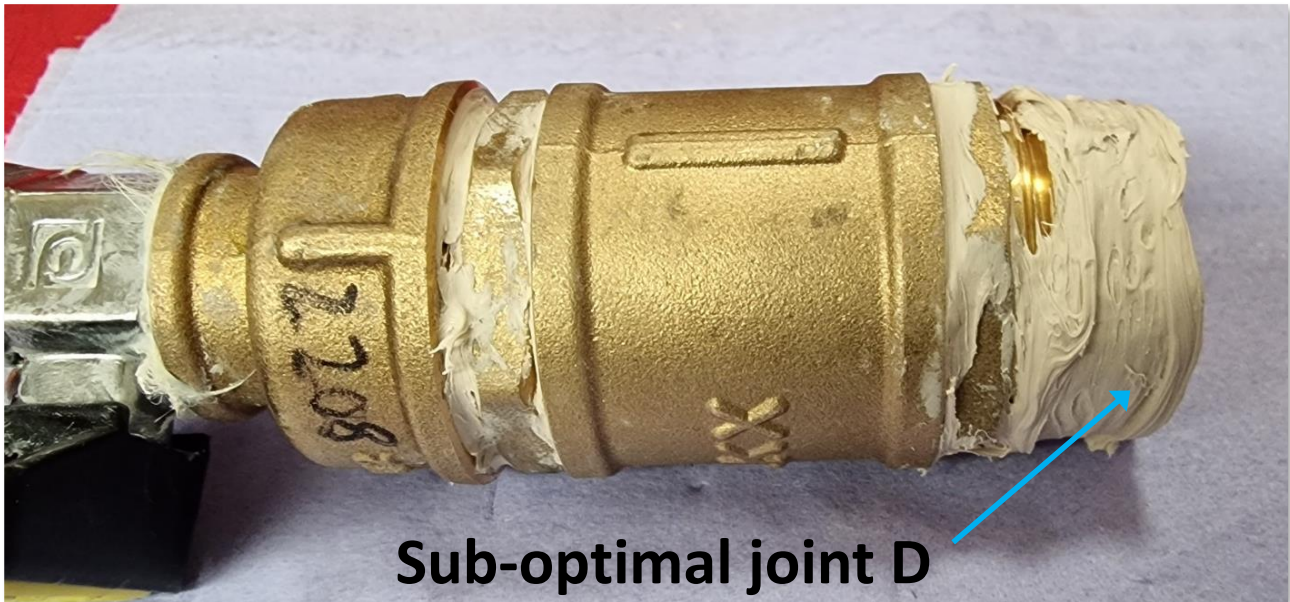
Figure 5: String 2208 during assembly, with excessive compound applied to joint D
