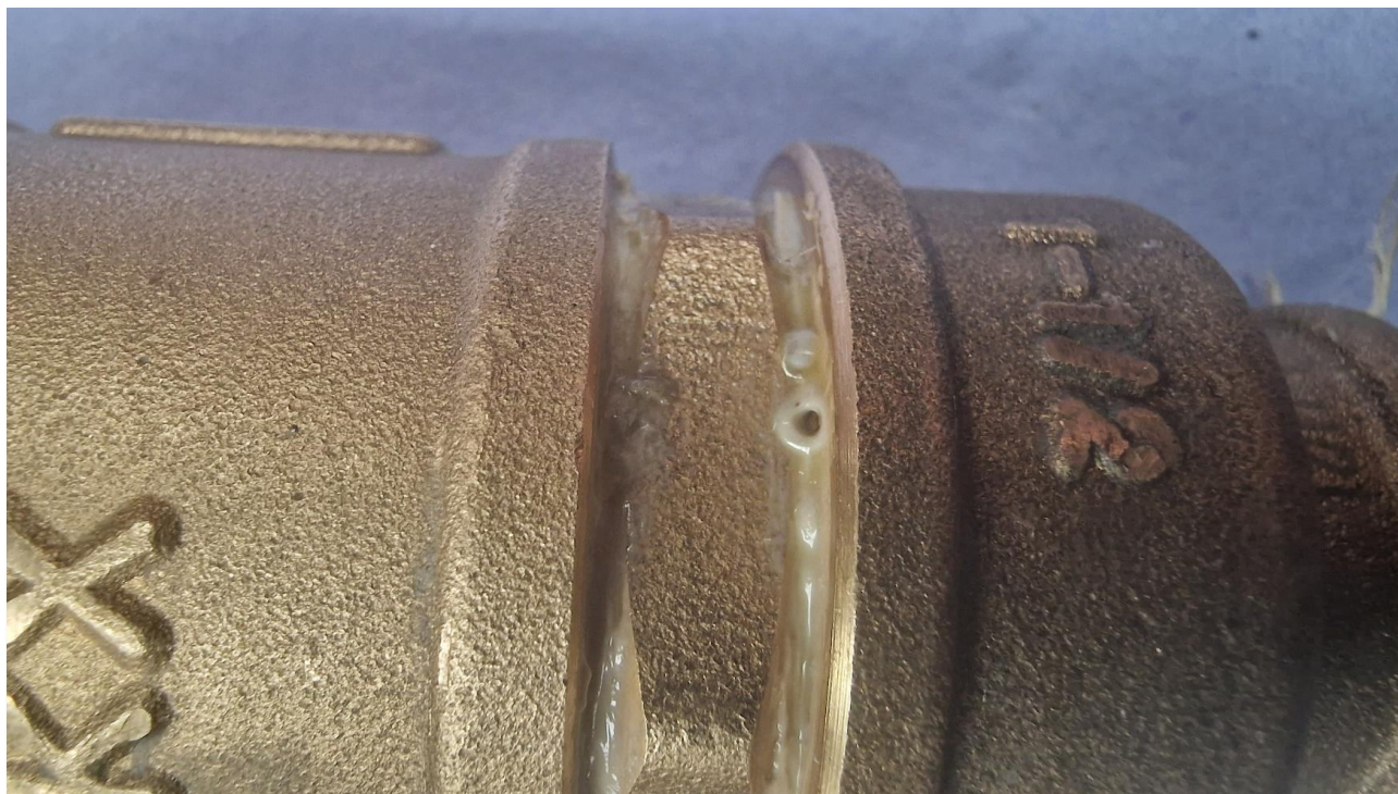
Figure 21: 6202 leak path after one week
