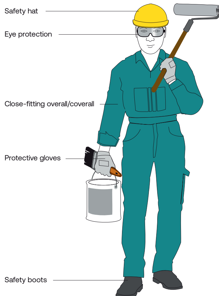
Figure 25.1 PPE for general painting
