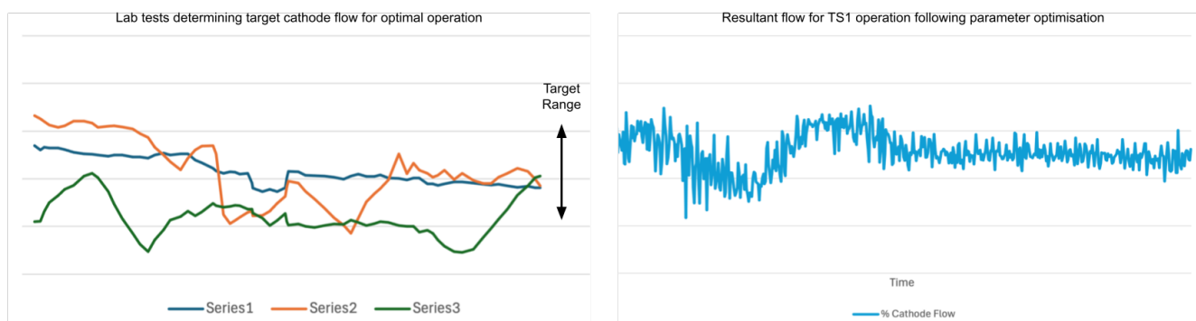
Figure 18 - Using lab parameterisation to define target operating range for TS1 (Right: lab, Left: TS1)
