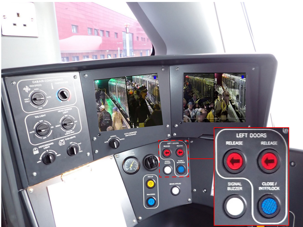
Figure 9: Still taken from the DOO CCTV recordings, superimposed by RAIB onto a photograph of the monitors in the driver's cab (photo taken during daylight hours).
