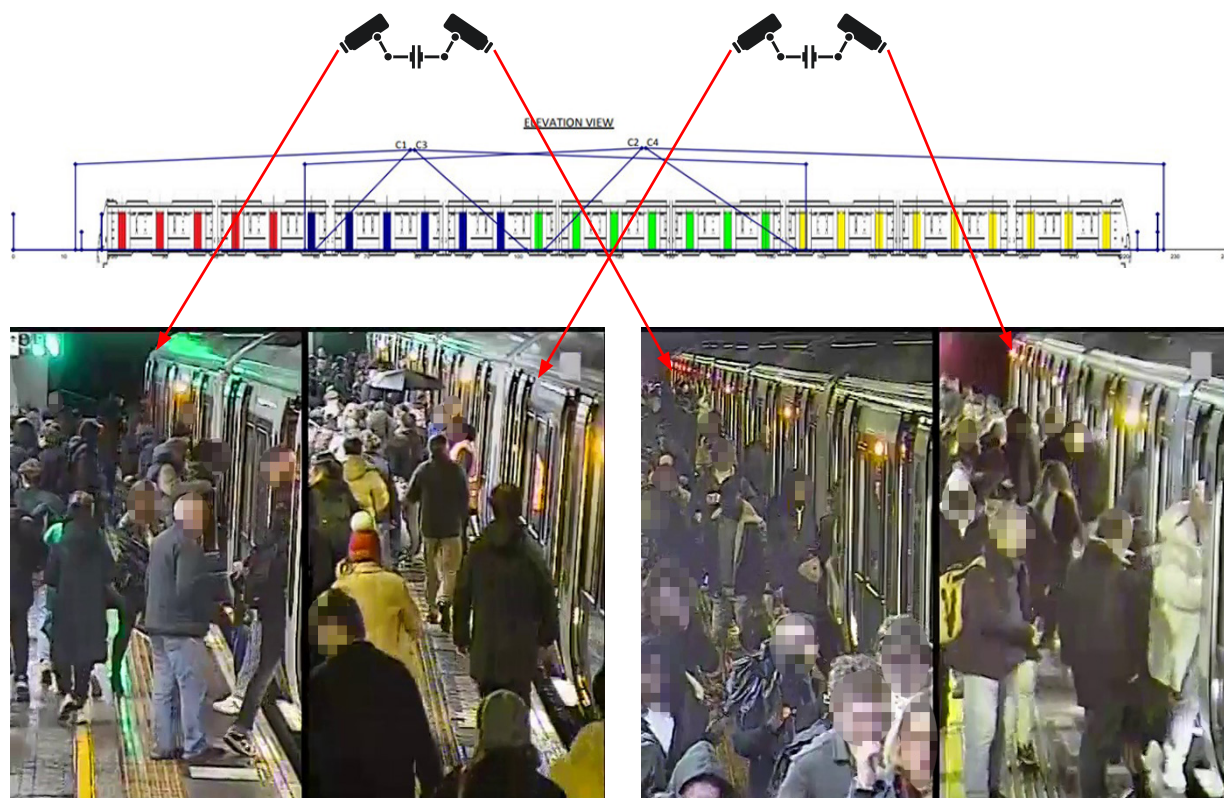
Figure 19: DOO camera positioning on platform 3 and actual view available to driver at 00:09 (images courtesy of MTREL).
