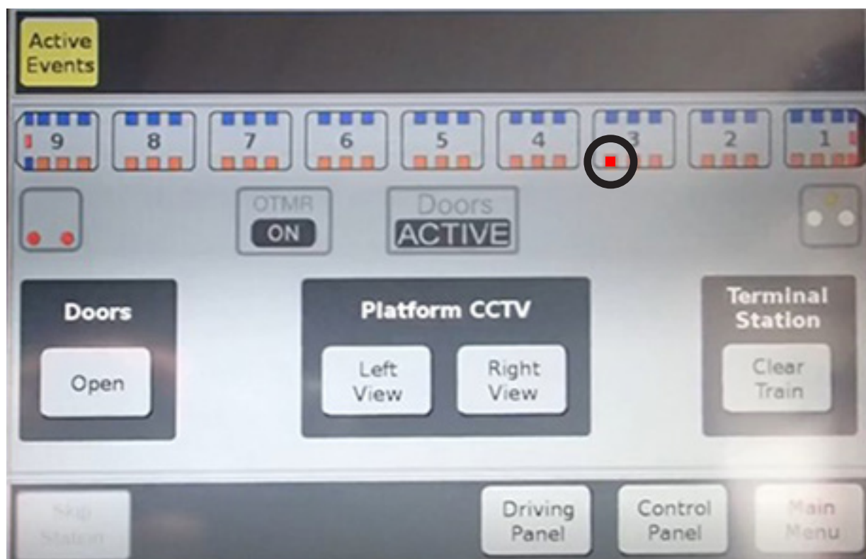
Figure 13: An example of a driver's panel displaying an item detected in the train's door.
