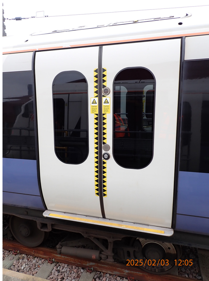
Figure 7: The class 345 electrically operated, sliding plug doors.
