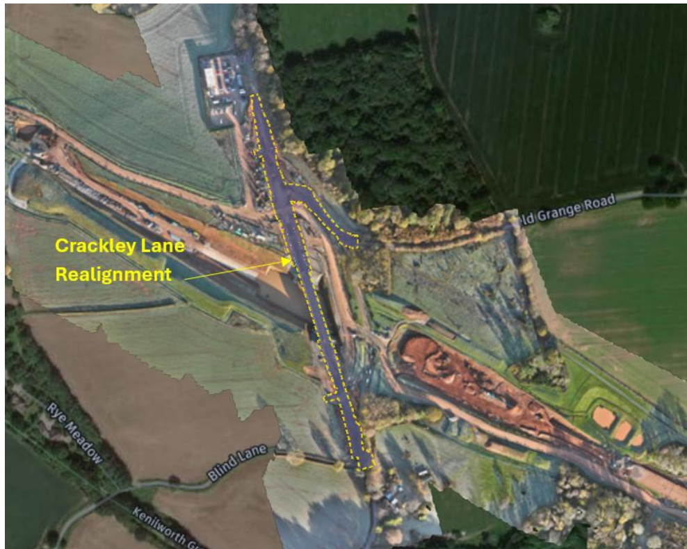
Figure 2 Post-HS2 highway network and associated construction works
