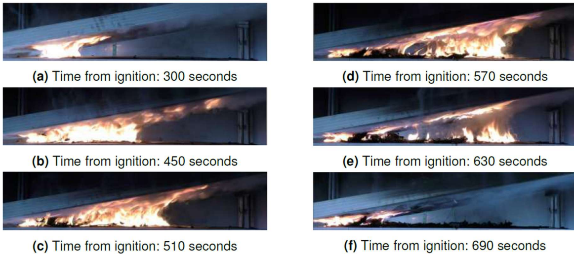
Figure 14. Flame spread on roof construction mock-up with mineral wool below the roofing membrane, a gap height of 8 cm, and an inclination of 10°, from (4).
