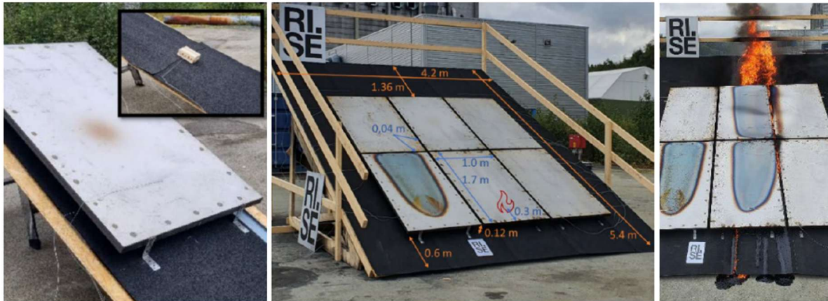
Figure 18. Medium-scale experiments with a wood crib placed on top of a roofing membrane with a steel plate (left) and without a steel plate (left inserted). Large-scale experiment with steel plate on a roof measuring 4.2 × 5.4 m (middle). Fire propagation in large-scale approximately 20 minutes after ignition where the fire has spread up to the top of the roof (red arrow) and down to the lower edge in the flowing melted bitumen roofing membrane (white arrow) (right), extracted from (13).
