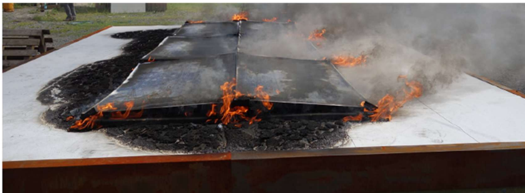
Figure 10. Experiment T3 from (11). The whole area underneath the PV array was affected by the fire, (11).
