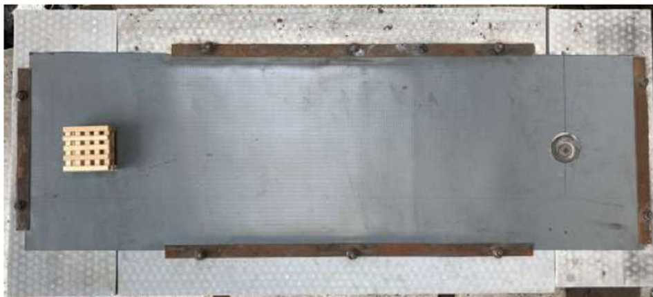
Figure 15. Top view of the mock-up roof construction before ignition of the wood crib. The wood cribs were made of pine sticks with a length of 81 mm and a squared cross-section with a side length of 9 mm, from (4).
