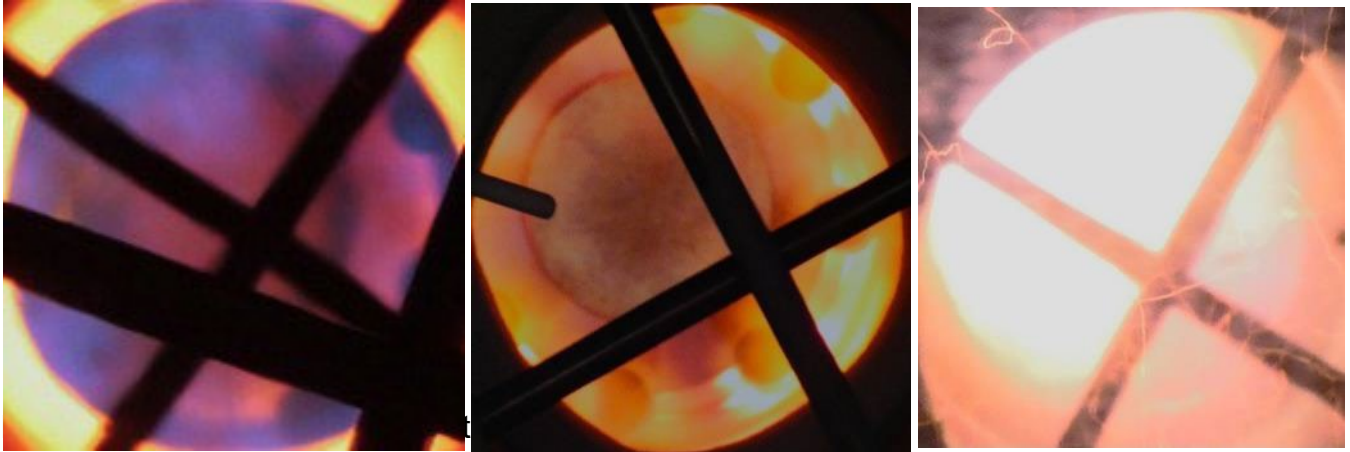
Figure 11. Jet Mix burner operating at 1 MW on NG (LHS), hydrogen (Middle) and BGG (RHS).
