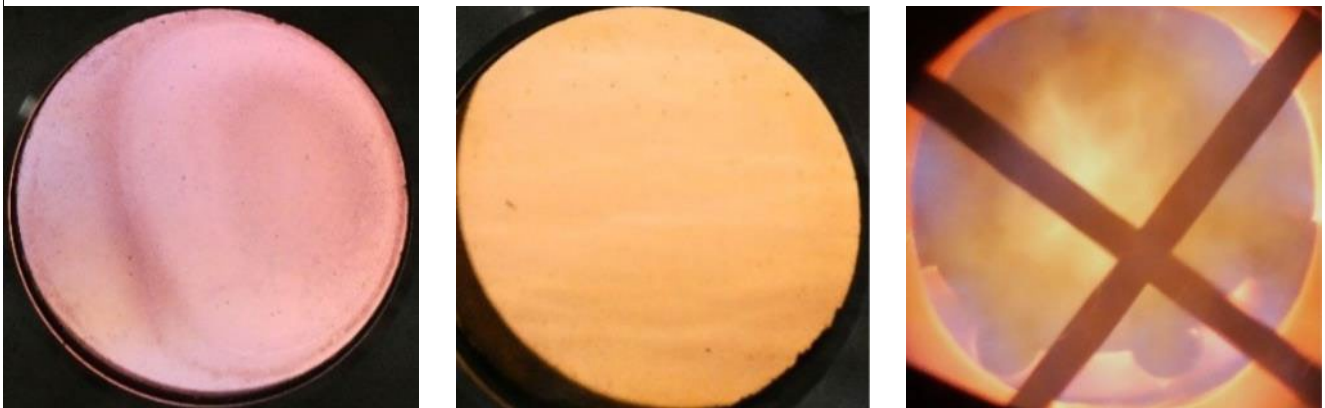
Figure 16. LHS- BGG flame close to BGG outlet; Middle – second stage flame ; RHS - Exit view of the BGG flame just after the NG was switched off. 320°C gasifier outlet temperature.
