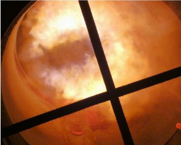
Figure 21. End flame view 45 mins after Figure 20 and 145 mins from the preburner ignition. The gasifier was at 500 deg C and the oxygen from the gasifier was 1.4%.
