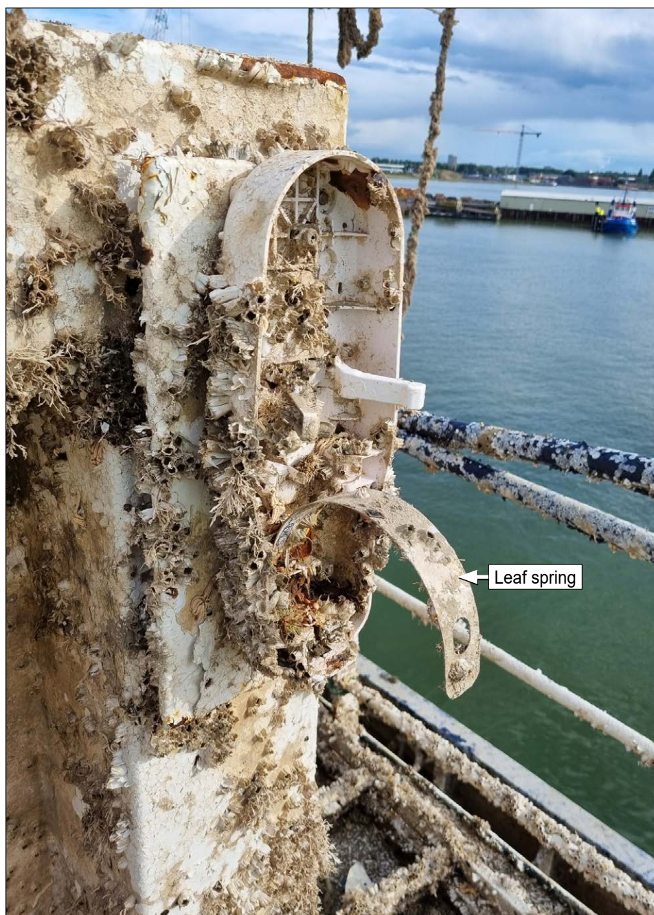
Figure 15: EPIRB housing with cover missing and ejection leaf spring deployed
