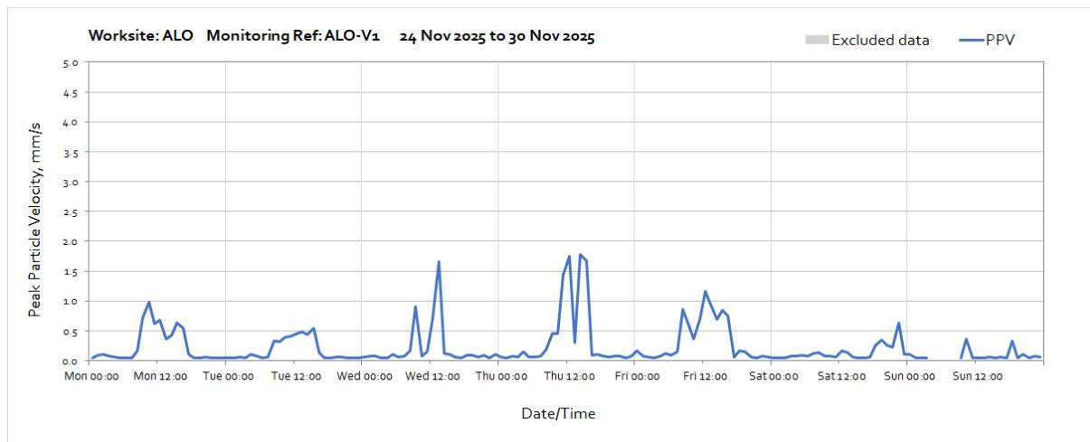
Note: Missing data throughout the week was due to a loss of power to the monitoring station caused by poor weather conditions preventing sufficient light reach the solar panel.
