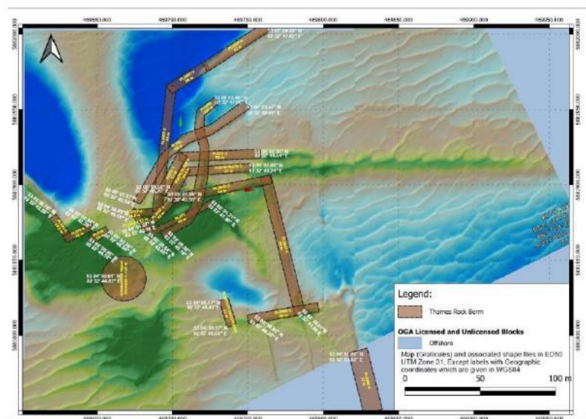
Figure 2.2 – Rock placement Thames Complex Area post-remediation
