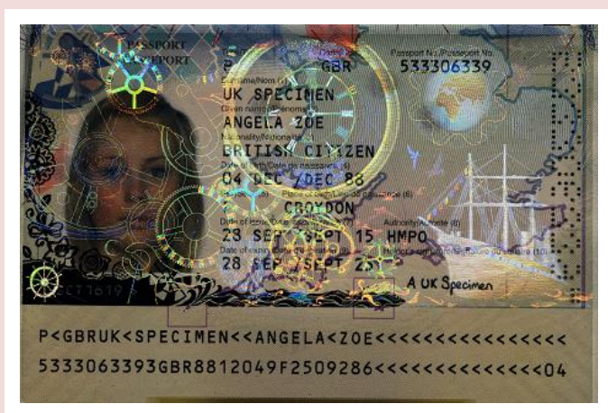
Holographic elements of thin film patch
