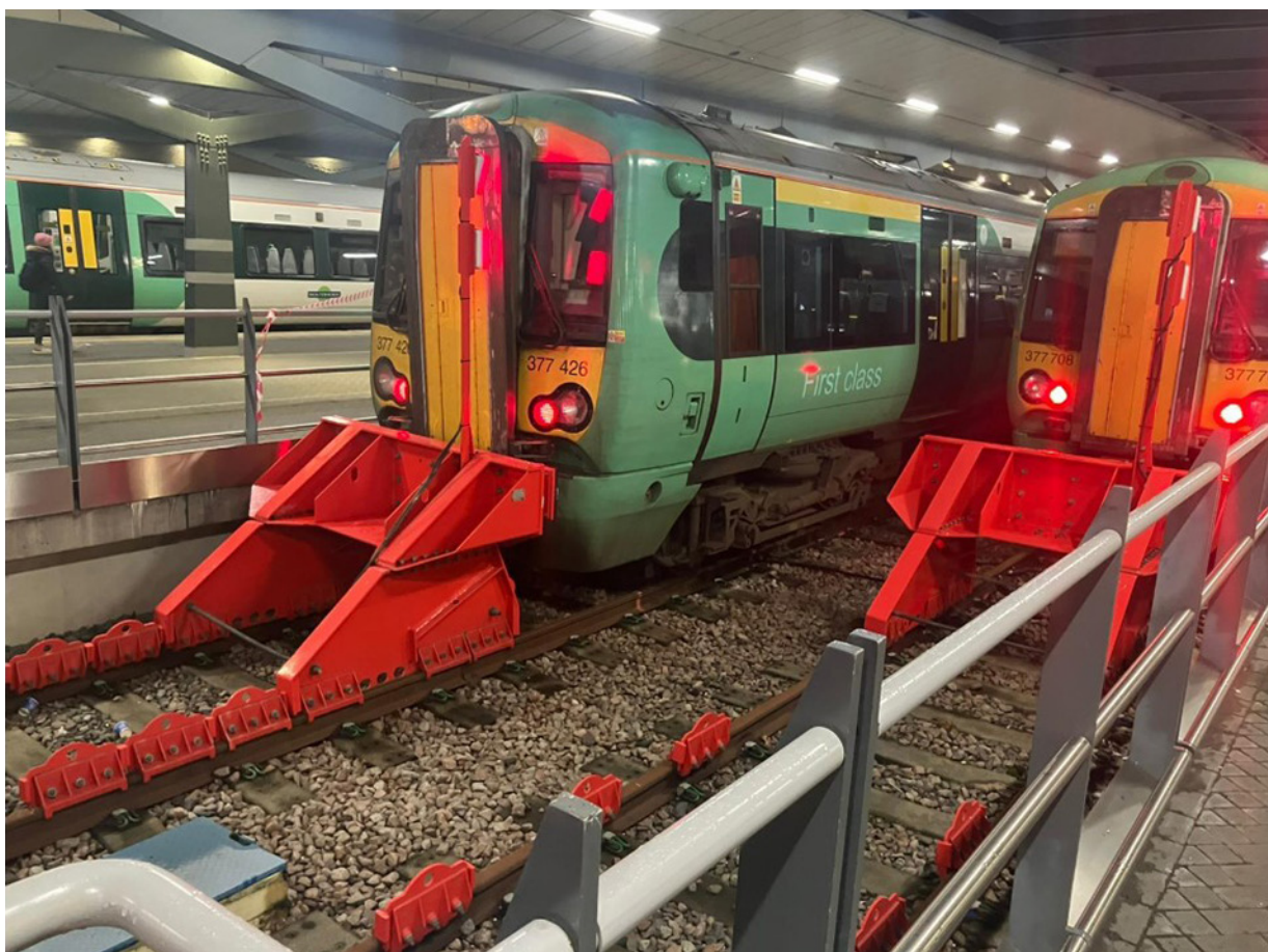
Figure 2: View of train 2F40 after it collided with the buffer stop at platform 12.
