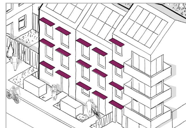
Fig 13 C4 Overheating and thermal comfort: Solar shades to minimise unwanted solar gain
