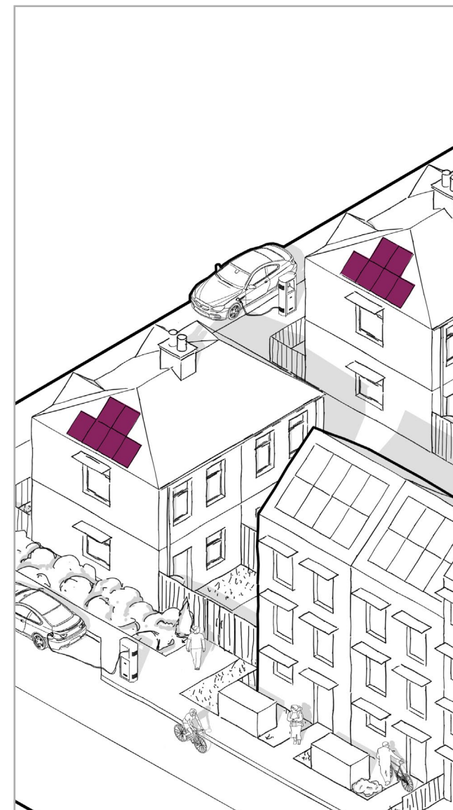
Fig 10 C1 Energy hierarchy: Maximise opportunities for solar PV generation with south facing roofs
