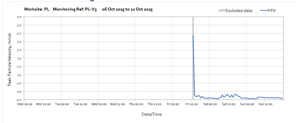
Note: Missing data between the start of the month and 13:00 on Friday 10<sup>th</sup> October was due to an issue with the monitoring station cable.
