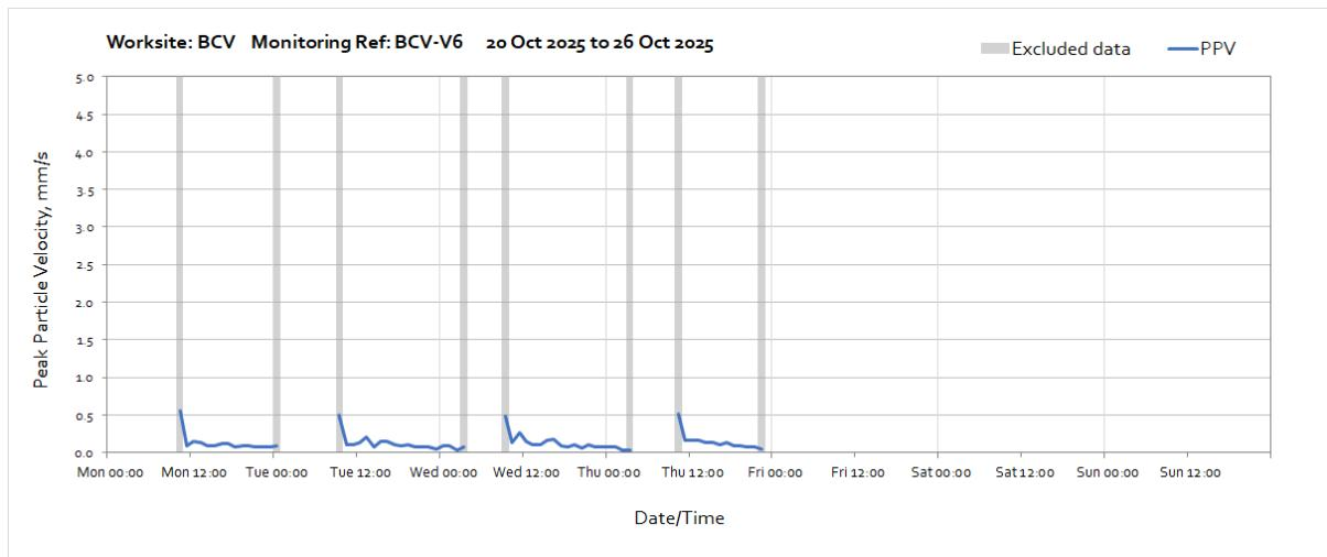
Note: Missing data throughout the month was due to a loss of power to the monitoring station caused by poor weather conditions preventing sufficient light reaching the solar panel.
