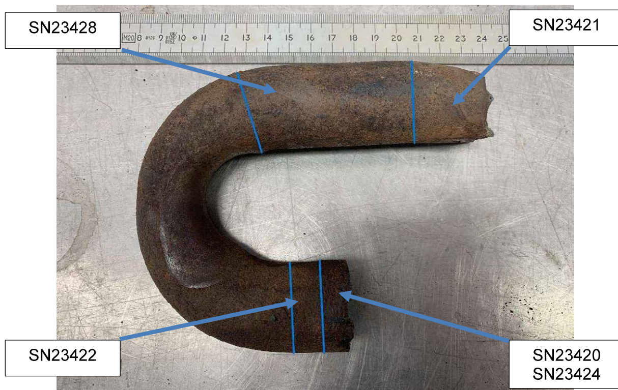
Figure 18: Partial chain link, sample 23307 (image 20240625_085251957_iOS modified to show sample locations)
