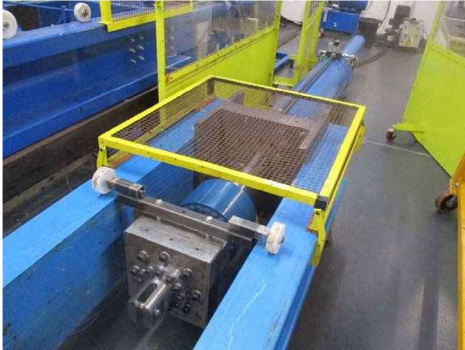
Figure 3.1: Main actuator 1.5 MN testing machine at TTI Testing's laboratory in Wallingford, UK. The load cell is just behind the tooling plate on which is mounted one of the chain fittings.
