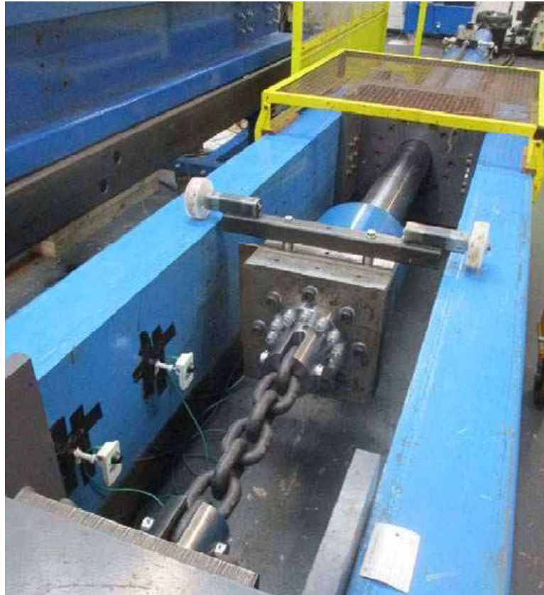
Figure 6.3: Test 2 sample set up in the 1.5 MN machine with new test fittings.
