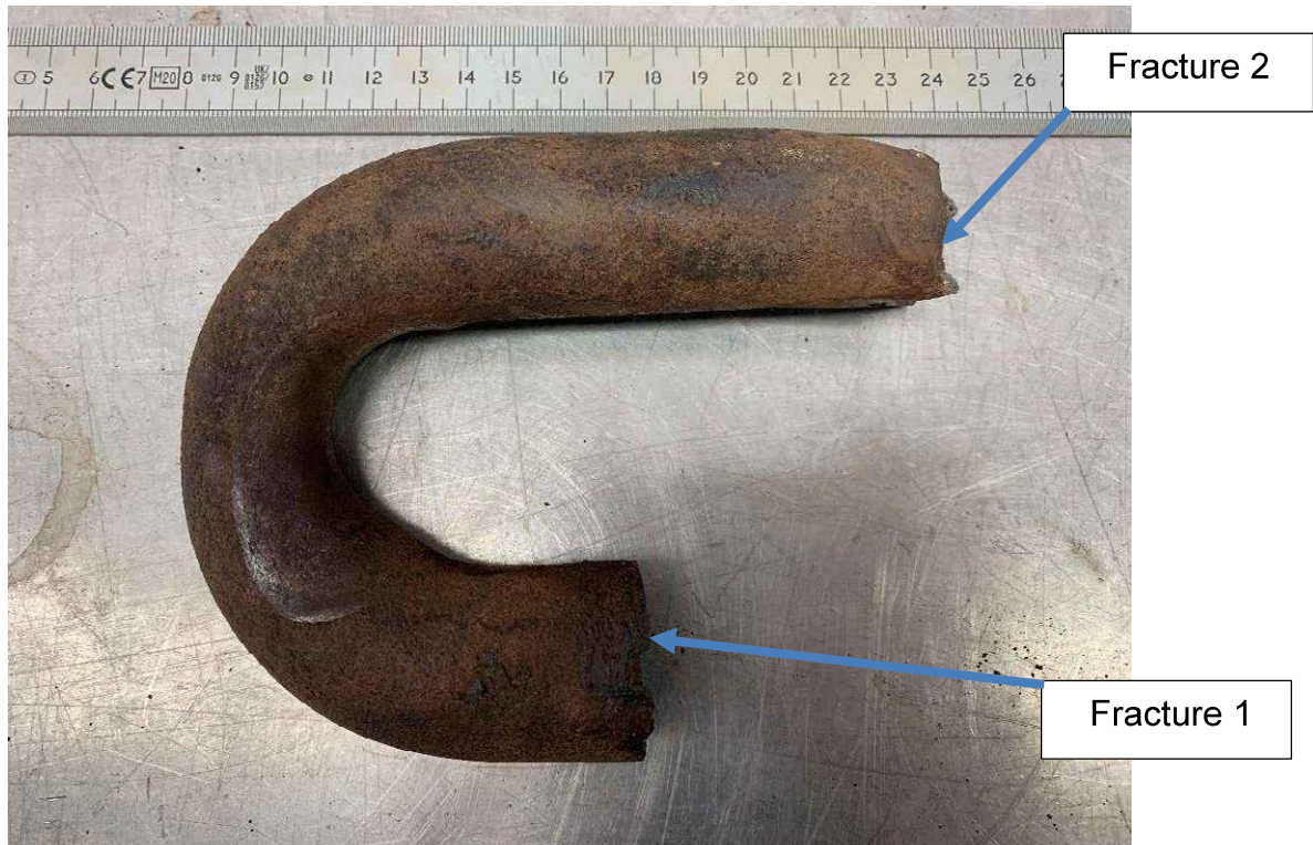
Figure 3: Partial chain link, sample 23307 (image 20240625_085251957_iOS)
