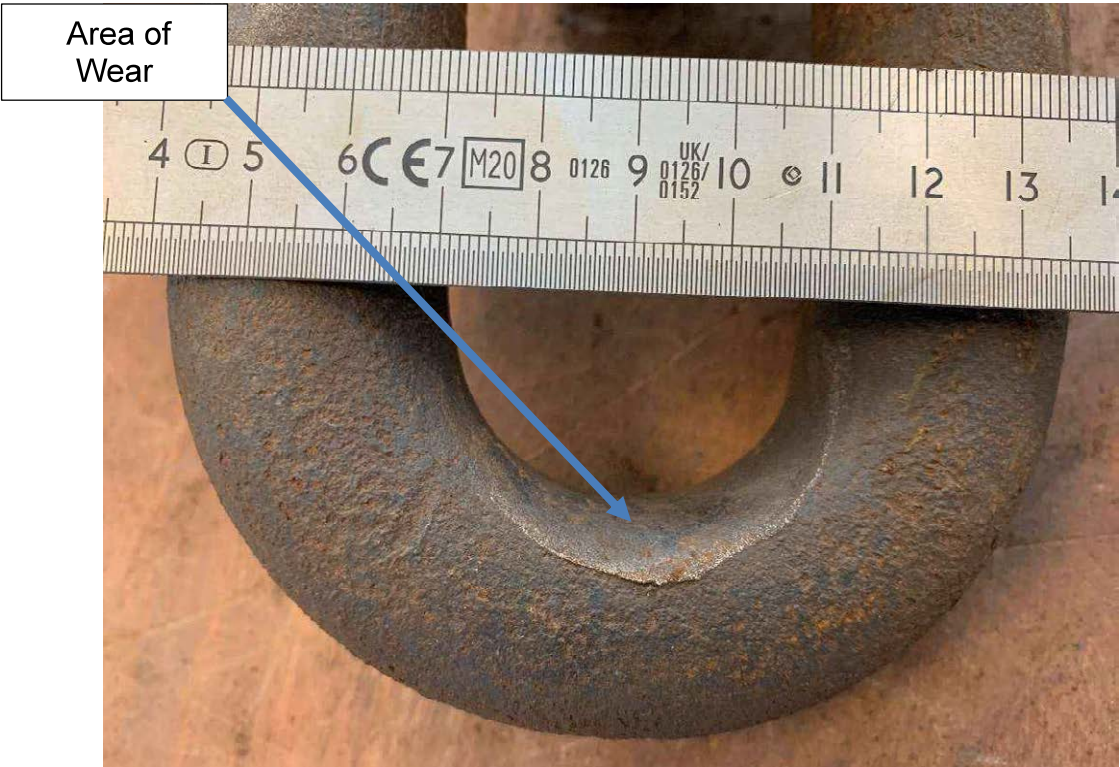
Figure 15: Wear on link 7 sample 23310 (image 20240621_103338363_iOS)
