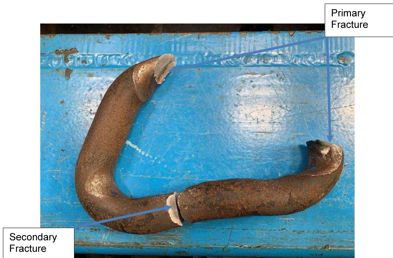
Figure 37: Samples 23544 & 23545 from 23309 post MBL test showing the fractured link (20241017_104856329_iOS)
