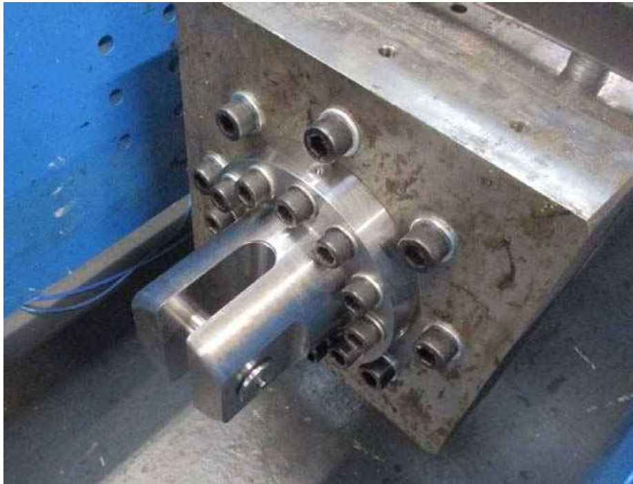
Figure 3.2: Ø32 mm chain fittings used for the first test.
