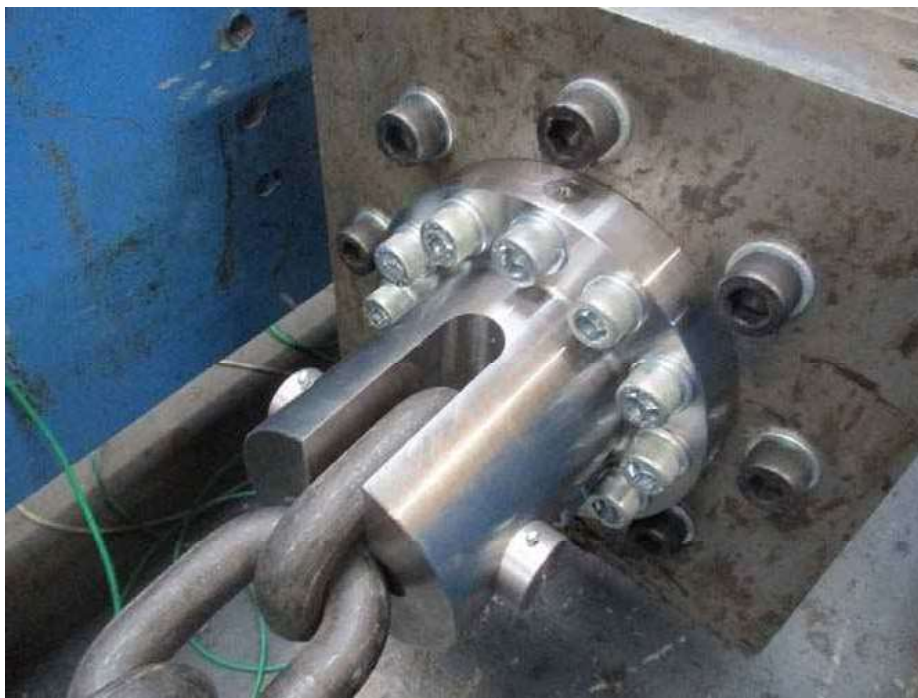
Figure 3.3: Re-designed Ø32 mm chain fittings used for tests 2 - 4.
