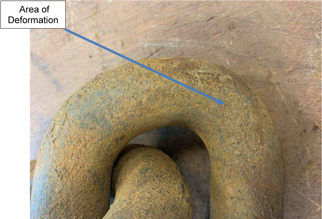
Figure 11: Deformation on link 2 sample 23310 (image 20240620_151007950_iOS rotated)
