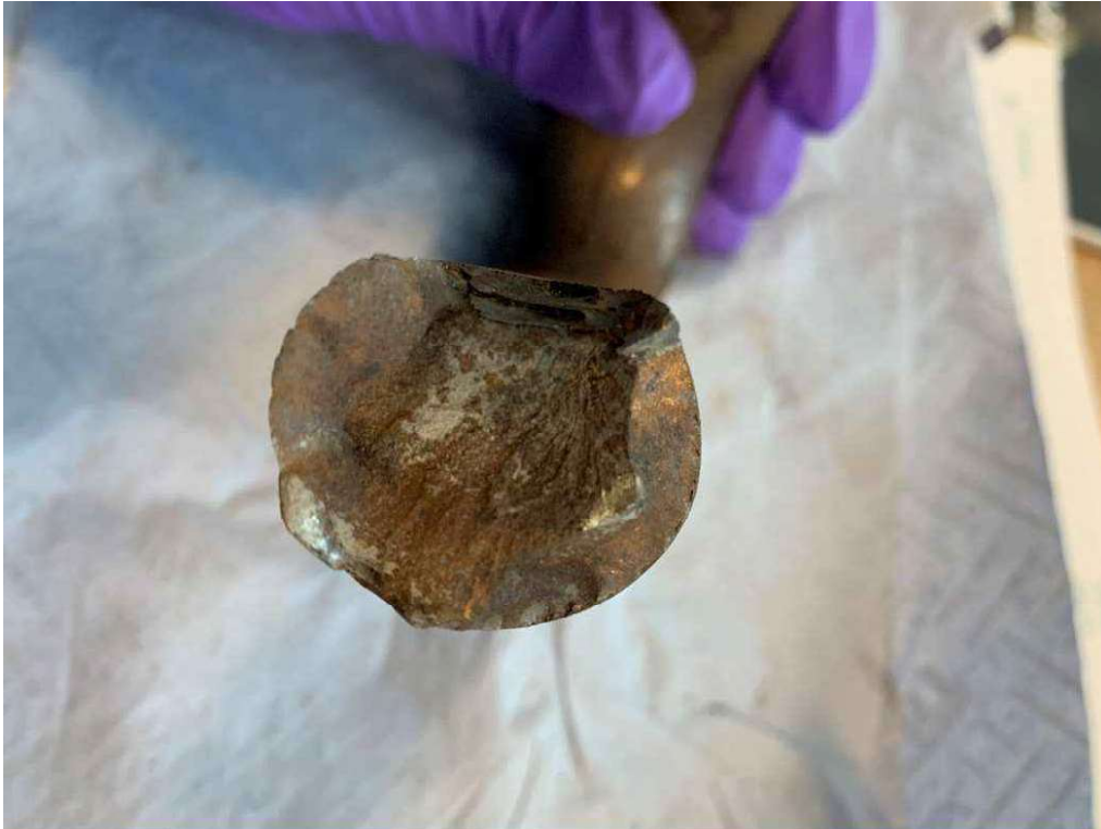
Figure 5: Partial Chain Link Fracture Face 2, sample 23307 (image 20240605_152047417_iOS rotated)
