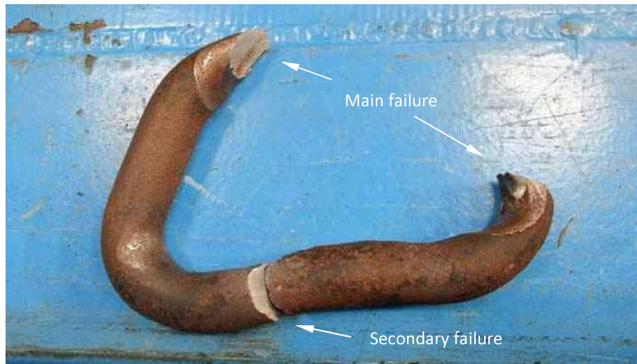
Figure 6.9: Failed link after testing of sample 23309 (Test 4).
