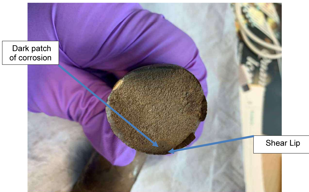
Figure 4: Partial Chain Link Fracture Face 1, sample 23307 (image 20240605_152035447_iOS rotated)
