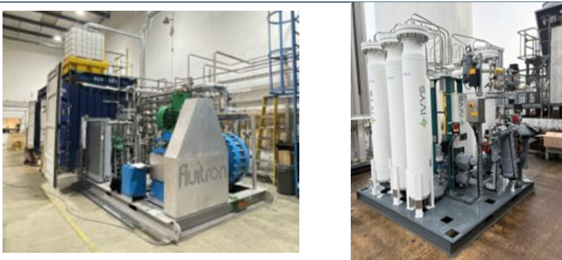
Figure 3.3: Compressor (left) and pressure swing adsorption unit (right)
