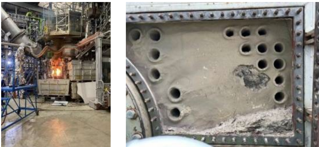
Figure 19 – Tapping the Furnace/Ash Build Up in Syngas Cooler
