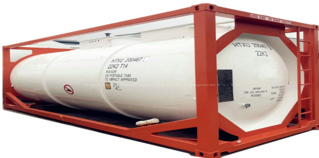
Figure 10: Ammonia iso-container delivery to site
