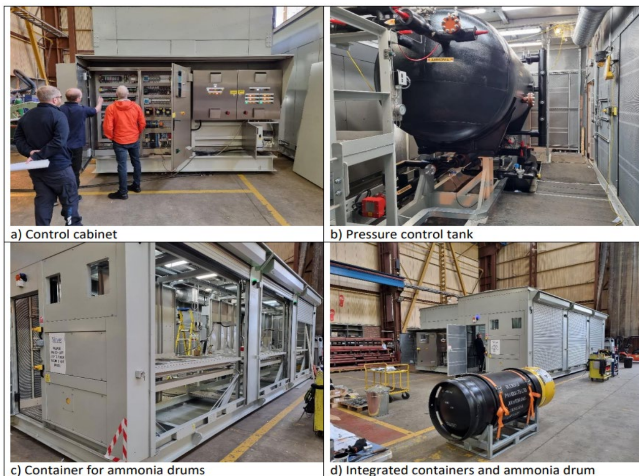
Figure 7: Ammonia decant and vaporisation units (unit 1 and 2)
