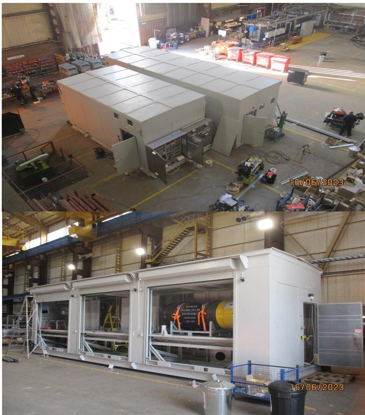
Figure 6: Ammonia decant and vaporisation units
