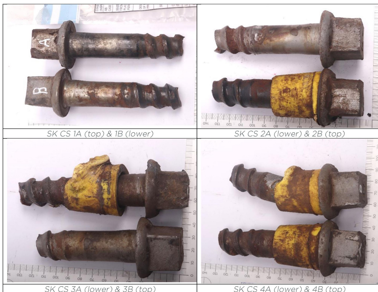
Figure 11: Examples of broken upper portions of screws before metallurgical examination.
