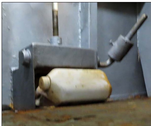
Figure 7: Example of a tonnage valve blocked by a loose object
