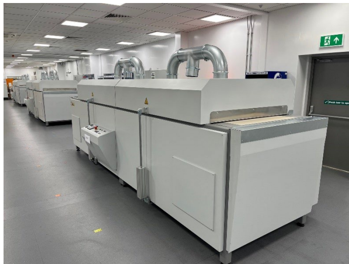
Figure 9: Phase 1 screen printing driers commissioned in Sheffield
