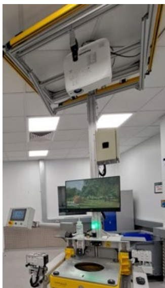
Figure 7: Stack assembly trolley with projector display and camera detection
