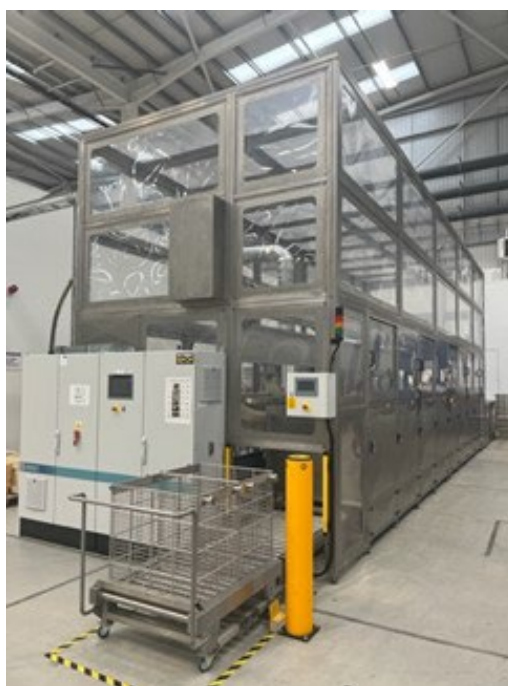
Figure 10: Automated washing and ultra-sonic cleaning set up in Sheffield
