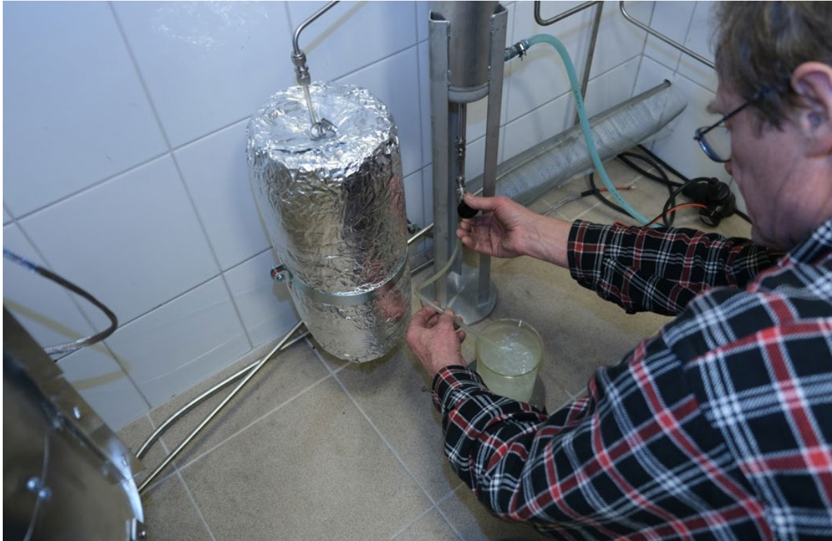
Figure A3-1 15 Collecting water product, in average 1200-1300 g from 20 min.
