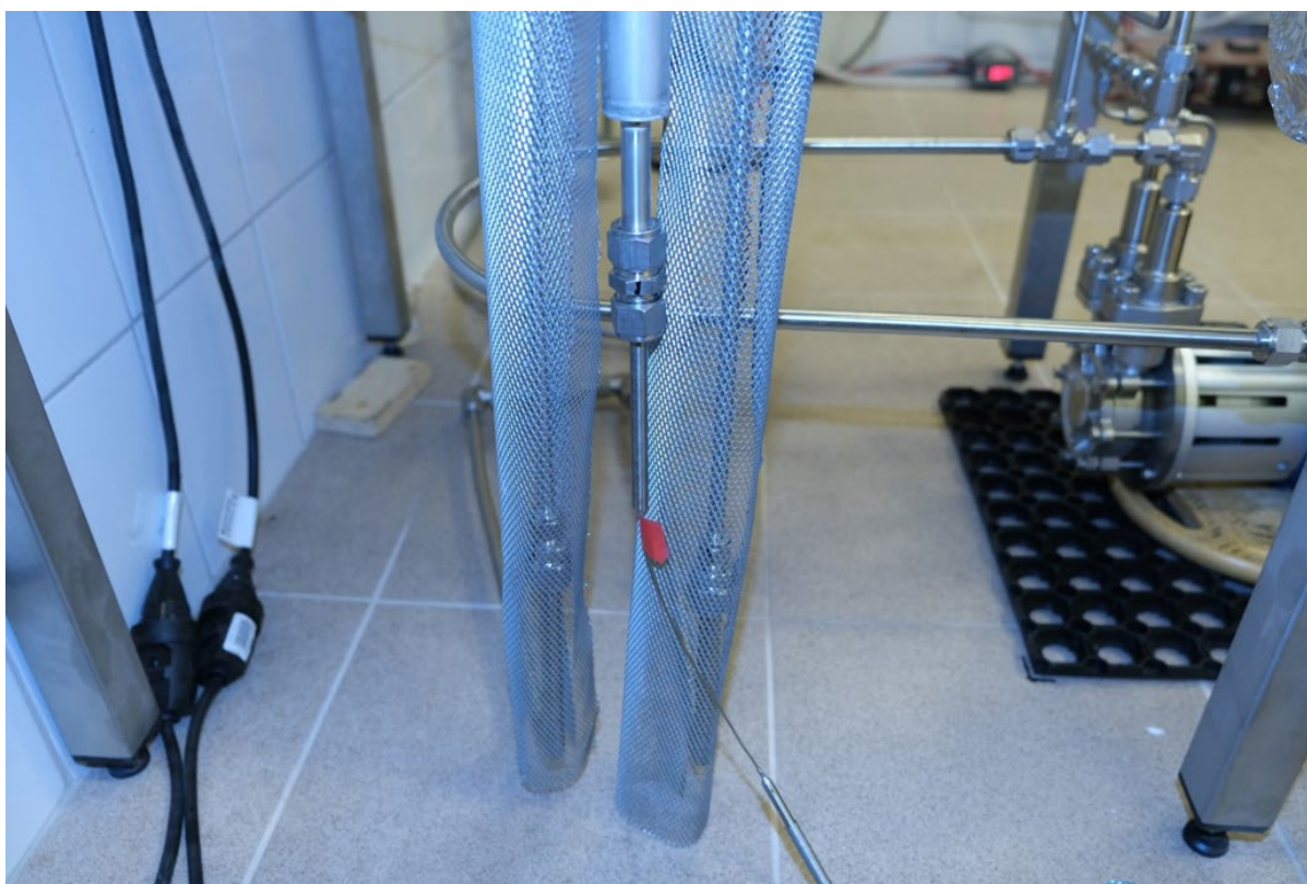
Figure A3-1 12 End of 2m long thermowell with sliding thermocouple
